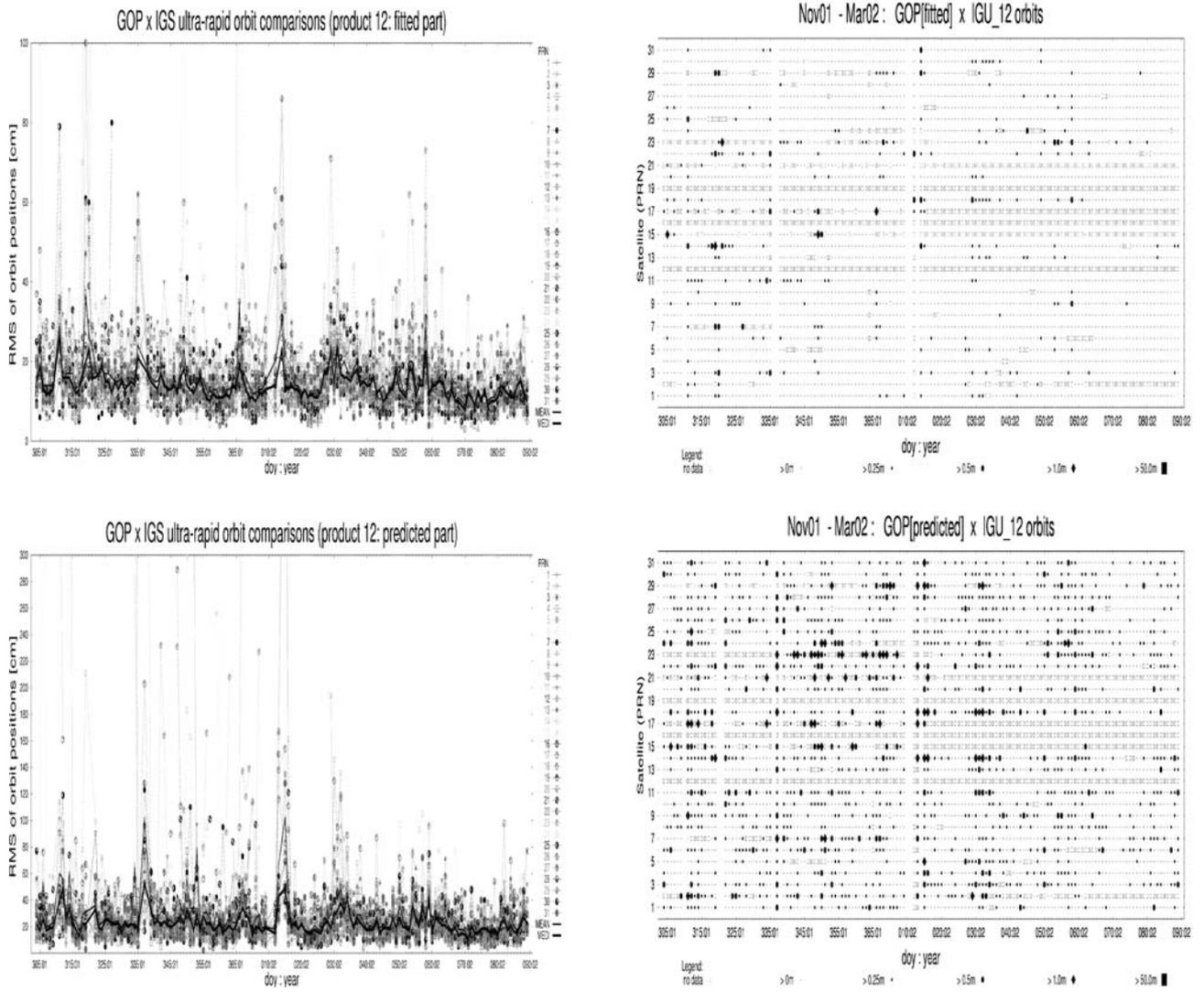
Figure 3. The comparisons between GOP and IGS ultra-rapid NRT orbits for fitted and predicted portions.
