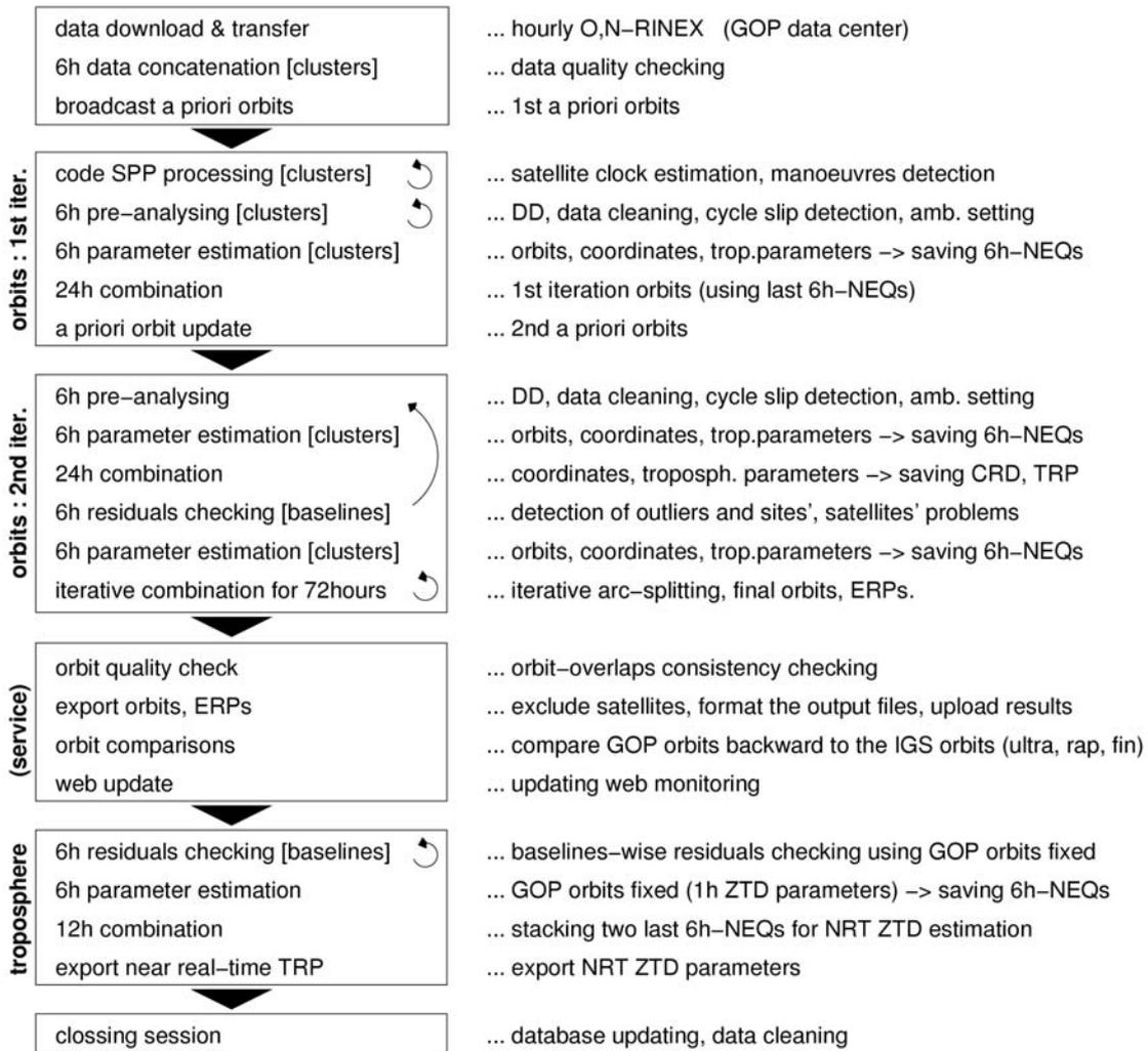
Figure 1. Analysing scheme of the GOP global NRT solution for the orbit determination and the tropospheric delay monitoring.
