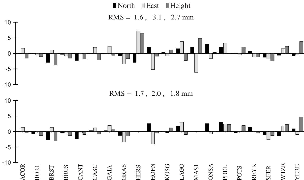
Fig. 6: Differences in north, east and height [mm] between the BERNESE and GIPSY/OASIS network adjustments and RMS values; top part: all stations included, bottom part: sparsely available stations HERS and MASI excluded
