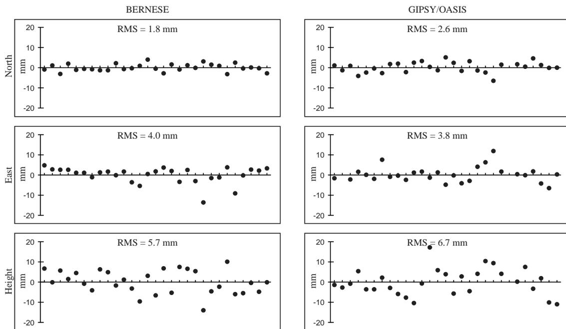
Fig. 5: Baseline BOGO-POTS fix solution daily; y repeatabilities in north, east and height with respect to mean [mm]
