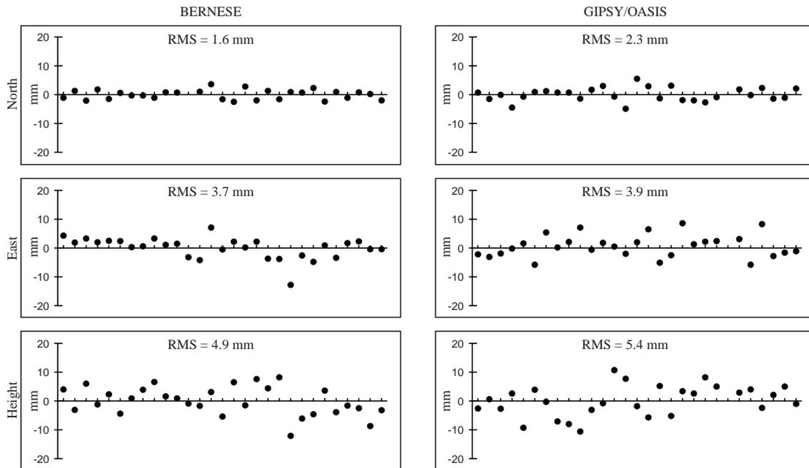
Fig. 4: Baseline BOGO-POTS float solution; daily repeatabilities in north, east and height with respect to mean [mm]
