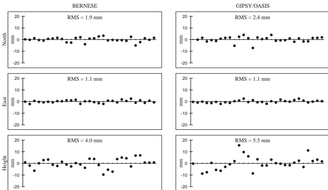
Fig. 3: Baseline POTS-BOR1 fix solution; daily repeatabilities in north, east and height with respect to mean [mm]
