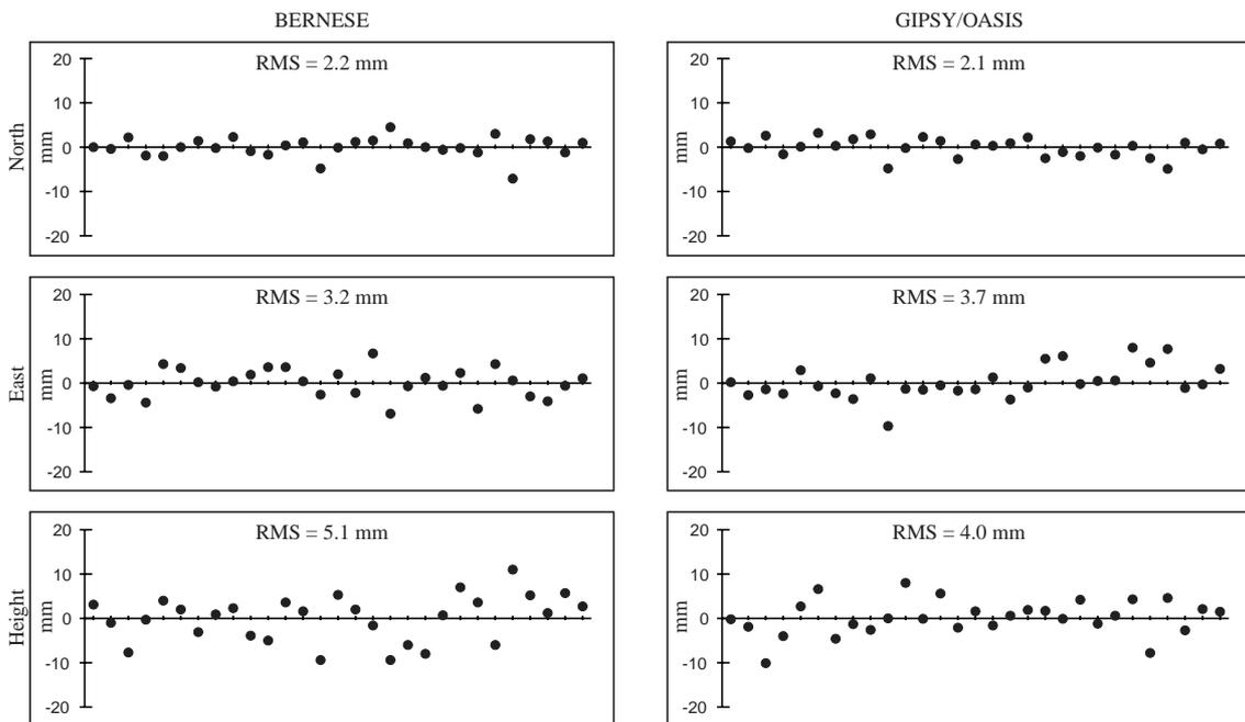
Fig. 2: Baseline POTS-BOR1 float solution; daily repeatabilities in north, east and height with respect to mean [mm]
