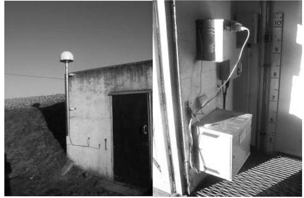
*Figure 4. Typical network RTK installation*
