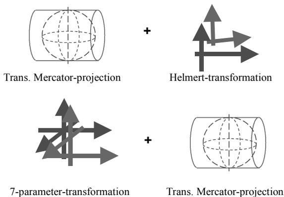
Figure 3. Different transformation combinations to handle rotated co-ordinate systems
