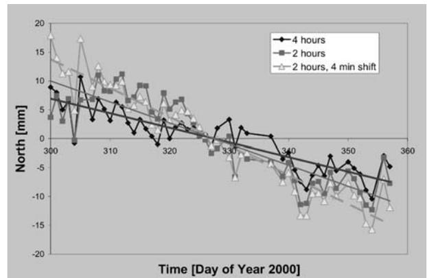
Fig. 7: Repeatability (north component) of the 3.7 km baseline ANDE-DMAN (section “B”) for L1 solutions based on a different selection of observation intervals (4 hours, central 2 hours, 2 hours shifted by 4 minutes every day)
