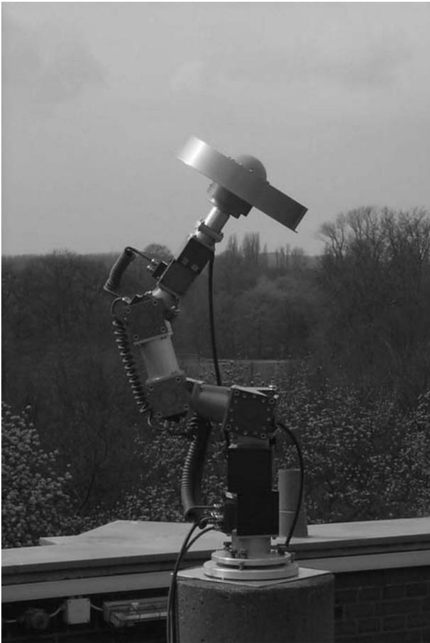
Figure 1: Robot for real time antenna calibration with test antenna.
