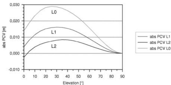
Figure 2: Elevation dependent absolute phase center correction for the Dorne Margolin AOAD/M\_T (L1, L2 and LC Signal) based on the IGS offsets.
