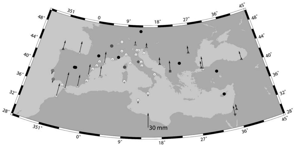
Figure 7: Apparent horizontal position changes caused by antenna domes
