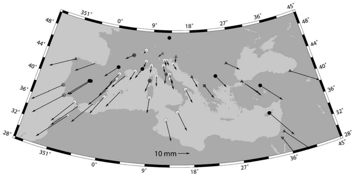
Figure 4: Apparent horizontal position changes caused by absolute PCV
