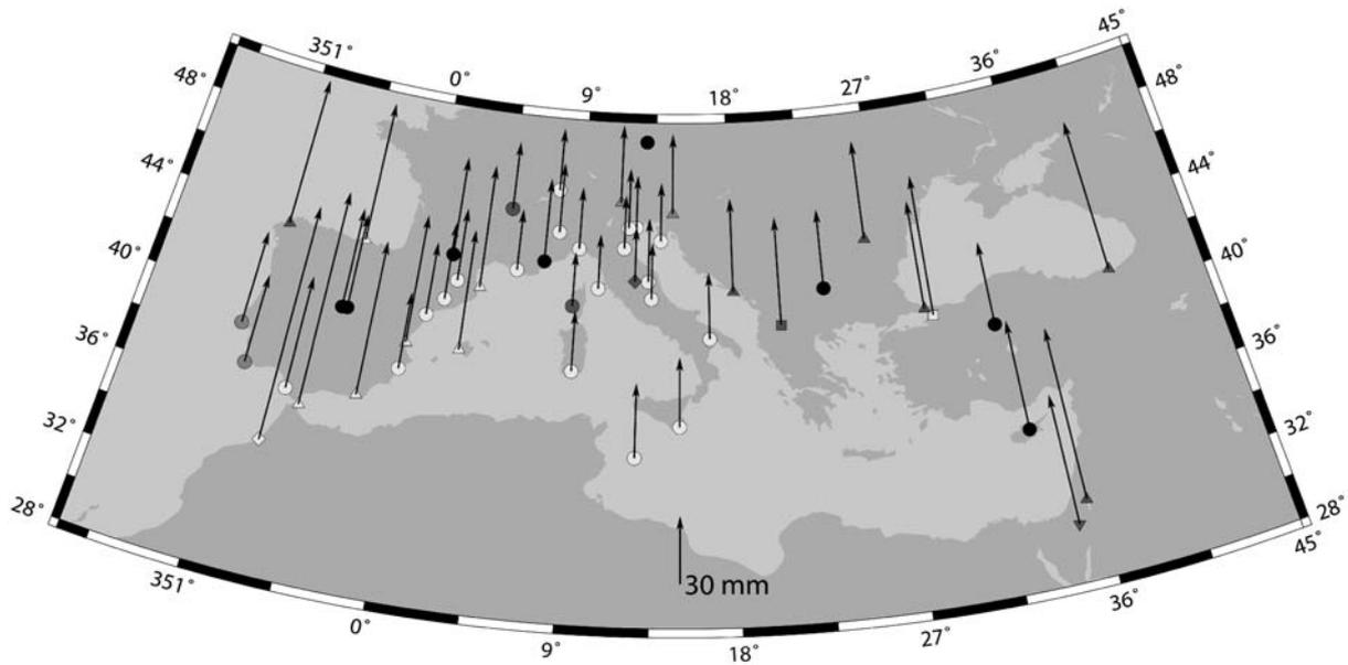
Figure 5: Apparent vertical position changes caused by absolute PCV
