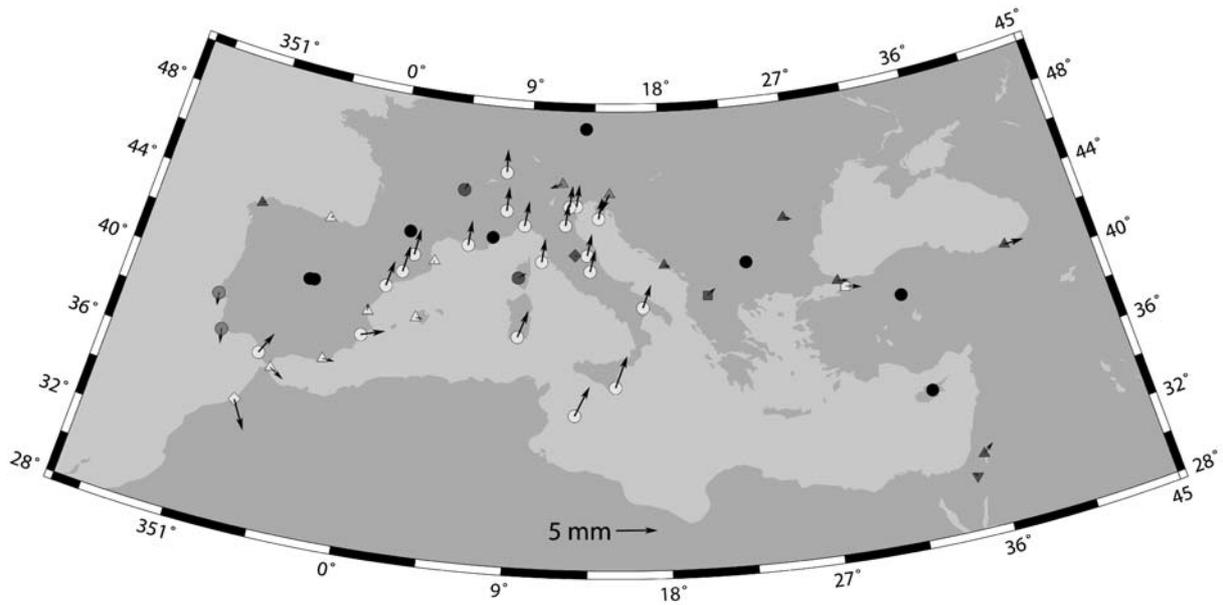
Figure 6: Apparent horizontal position changes caused by antenna domes
