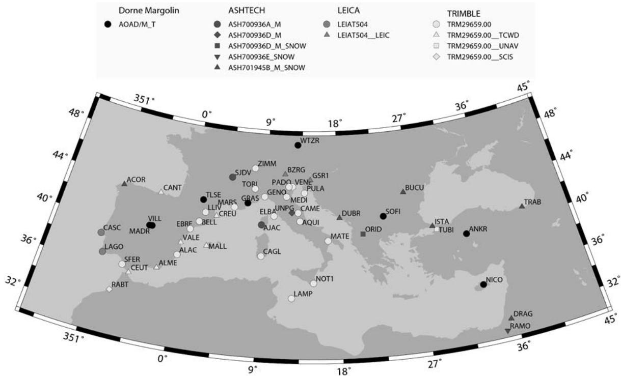
Figure 3: Map of the stations and antenna types used in the analysis
