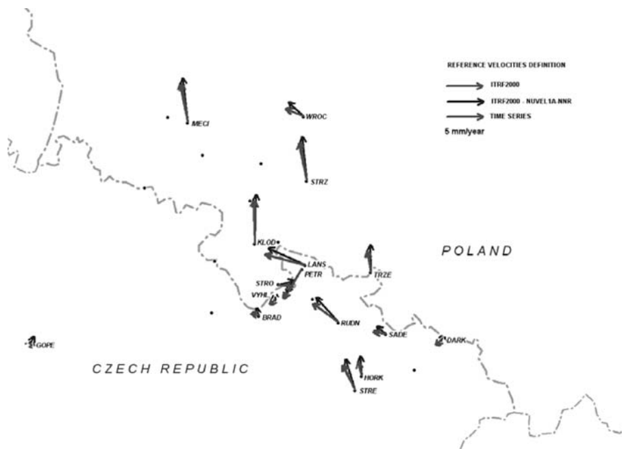
Fig. 10. Velocity vectors of the SUDETES network points – comparison of the approaches.
