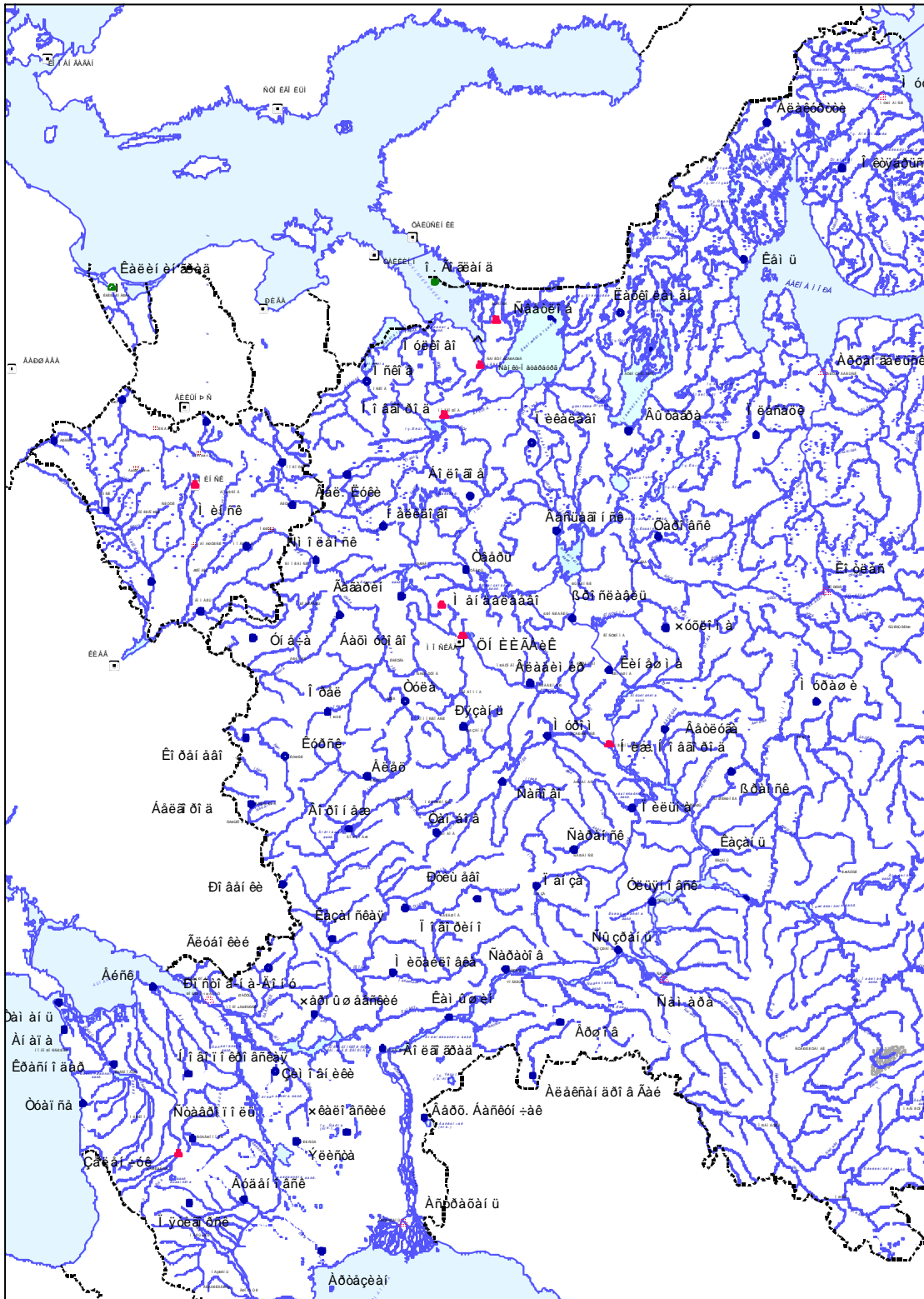
Fig. 1. Russian Reference Frame for the European territory (red points - fiducial GPS stations, blue and named dots - created points of the Precise Geodetic Network (PGN), green dots - planned points of PGN)
