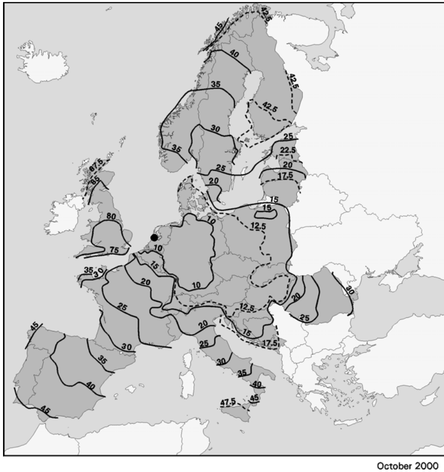
Figure 2: UELN 95/98 – Isolines of Precision [kgal × mm] (UELN-95/98 – extended for Estonia, Latvia, Lithuania and Romania)
