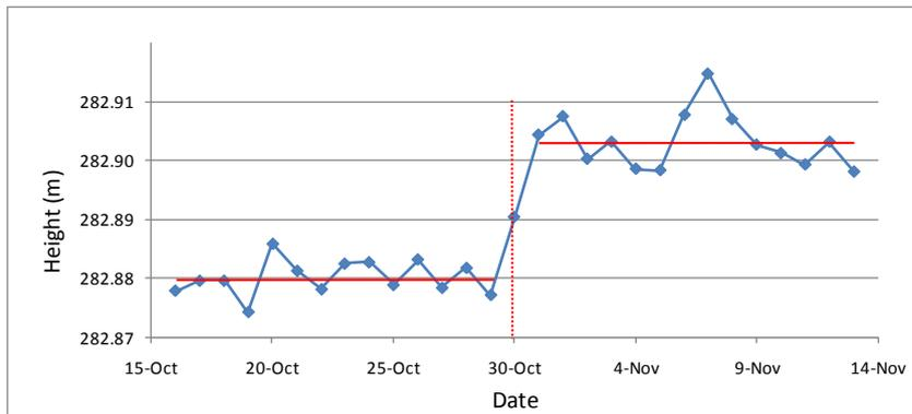
**Fig. 4** Time-series of height of station 093A (the vertical dashed line indicates the day of the earthquake).
