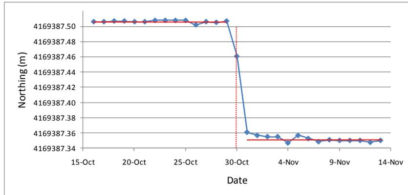
**Fig. 3** Time-series of Northing of station 093A (the vertical dashed line indicates the day of the earthquake).
