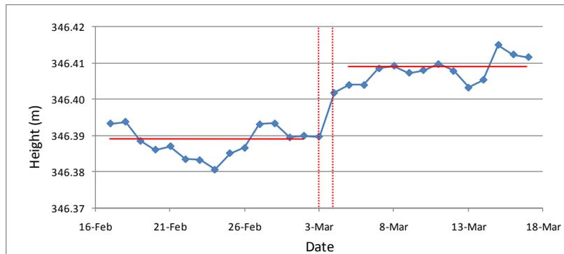
**Fig. 9** Time-series of height of station 057A (the vertical dashed lines indicate the days of the earthquakes).
