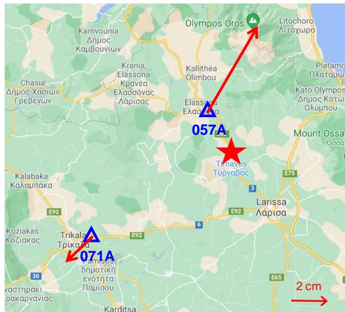
**Fig. 10** Estimated static horizontal displacements at nearby HEPOS reference stations. The epicentral area of the earthquakes is marked by red star.
