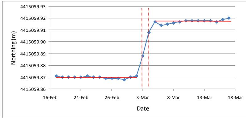
**Fig. 8** Time-series of Northing of station 057A (the vertical dashed lines indicate the days of the earthquakes).
