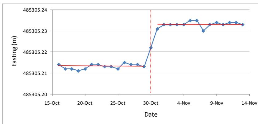
**Fig. 2** Time-series of Easting of station 093A (the vertical dashed line indicates the day of the earthquake).
