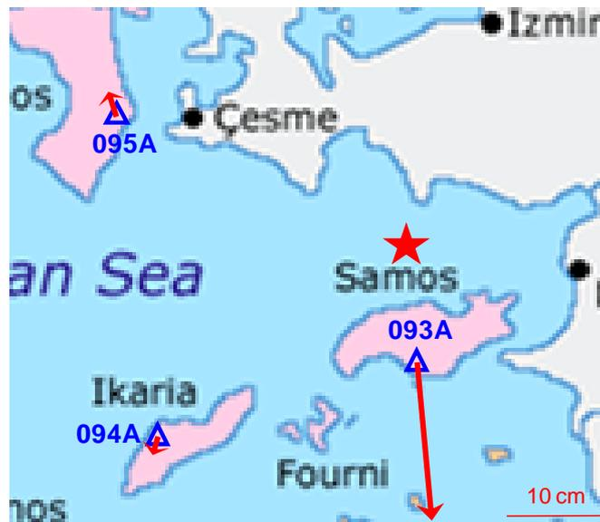
**Fig. 5** Estimated static horizontal displacements at nearby HEPOS reference stations. The epicenter of the earthquake is marked by red star.
