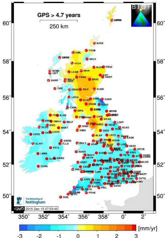
**Fig. 3** Map of current vertical station velocities at 162 CGPS stations in the UK, based on CGPS measurements for the period from 1997 to 2015:273
