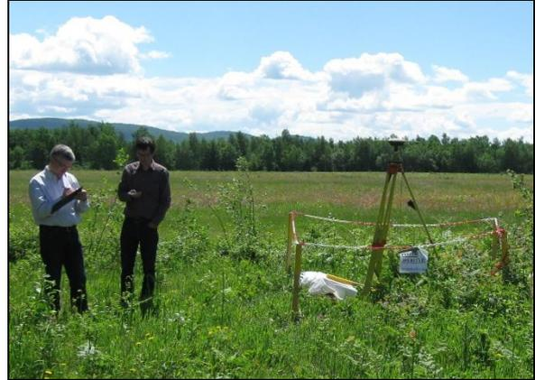
Figure 2: GNSS measurements at the location of the future Prilozje zero order network station.
