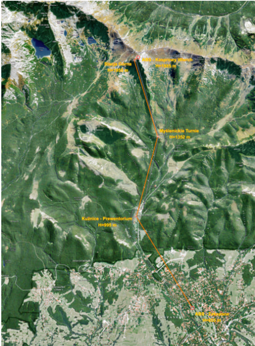
Fig. 11. High Mountains Calibration Baseline presented on the photomap of Polish part of Tatra Mountains elaborated in the Institute of Geodesy and Cartography in the scale of 1:20 000
