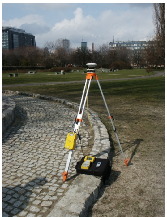
RTK Set with usage Trimble Data Controller Software
