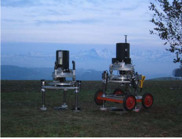
Figure 6: The two digital camera systems DIADEM (left: Zurich) and TZK2-D (right: Hanover)
