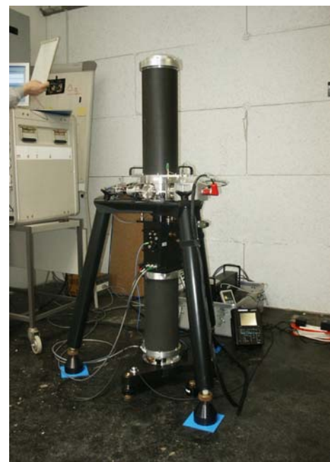
Figure 2: Absolute gravity measurements in Zimmerwald using an FG5
