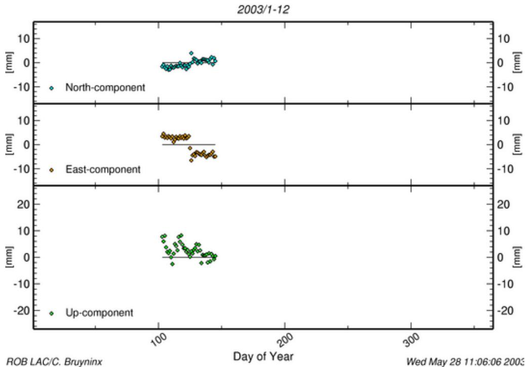
**Figure 10. Position time series computed for the PLRX site at the ROB.**
