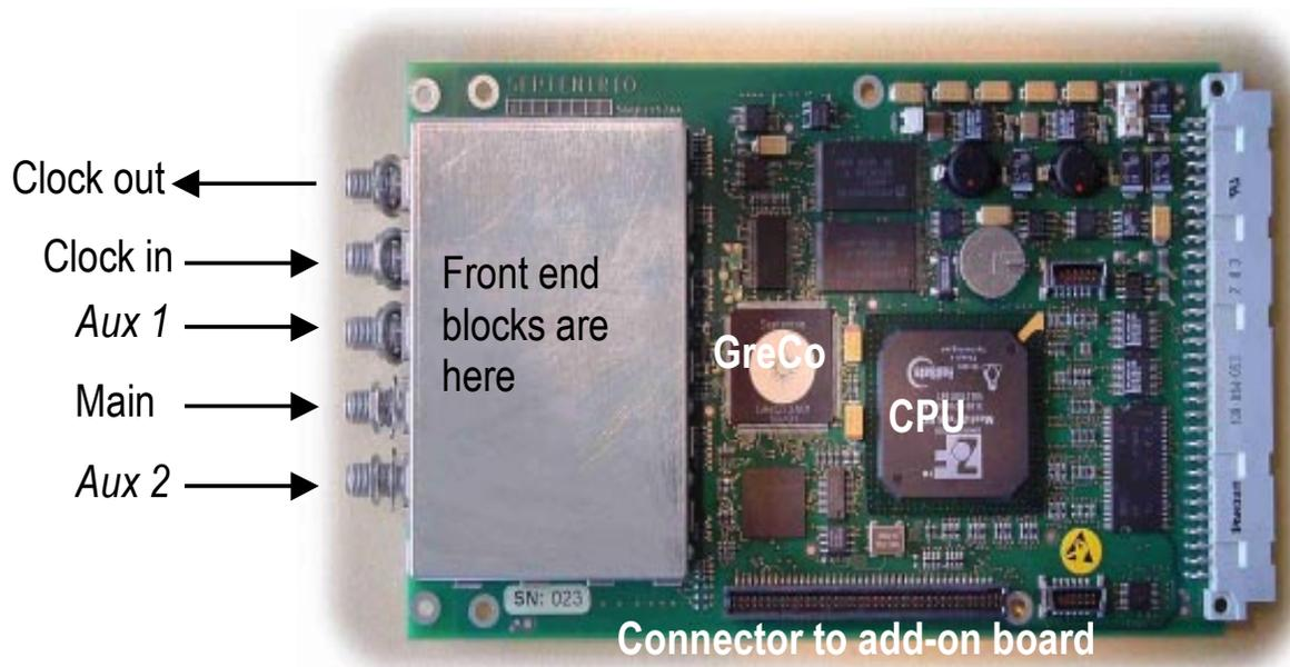
**Figure 3.** PolARx2 is implemented as a EuroCard-sized board. Additional RF input sockets are stipulated for auxiliary antennas (multi-antenna version only) and external clock reference for time transfer applications.
