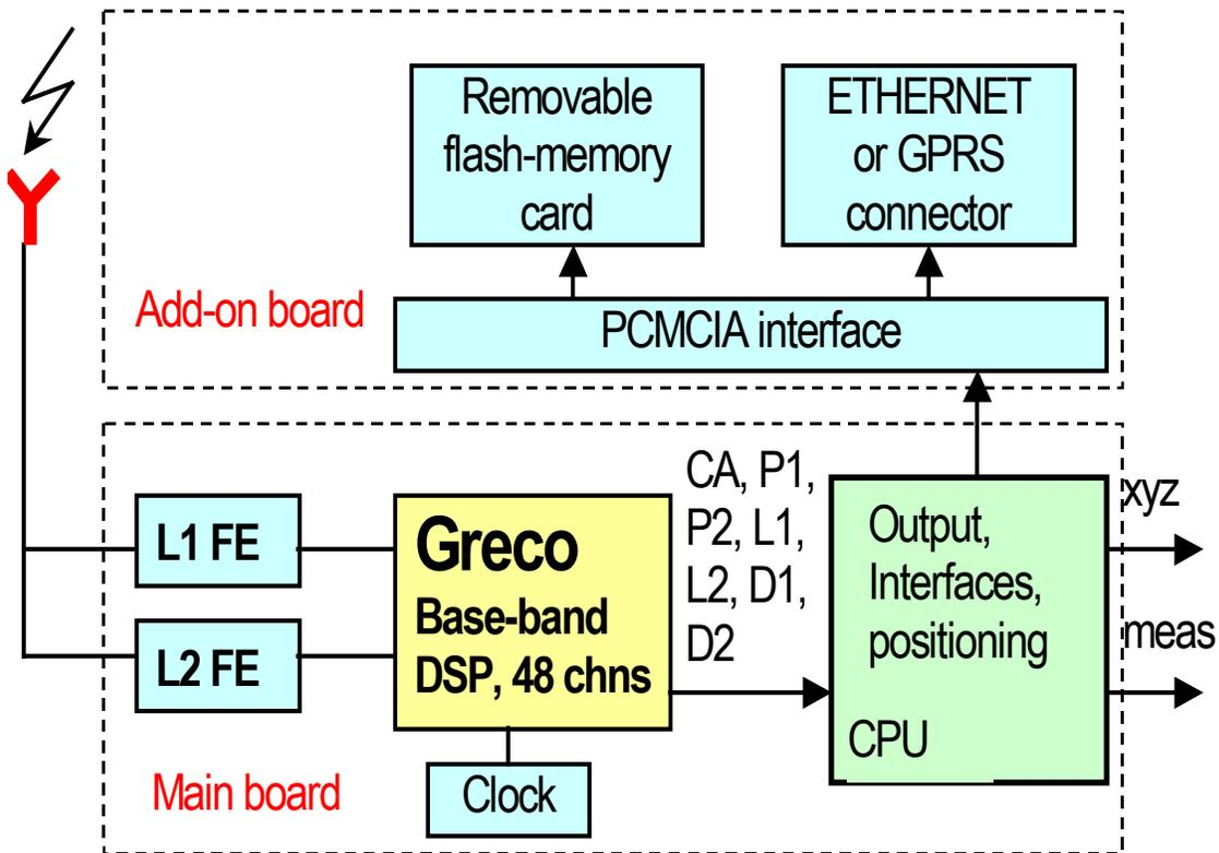
Figure 1. Hardware architecture of PolaRx2
