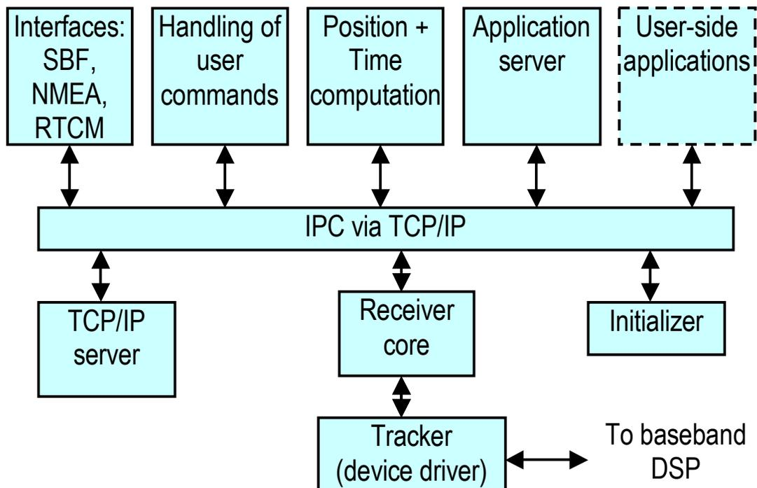
Figure 2. Software architecture of PolaRx2
