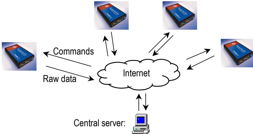
**Figure 7. New architecture of the data center application based on the TCP/IP connectivity of PolARx2. The central server runs multiple instances of RxControl.**
