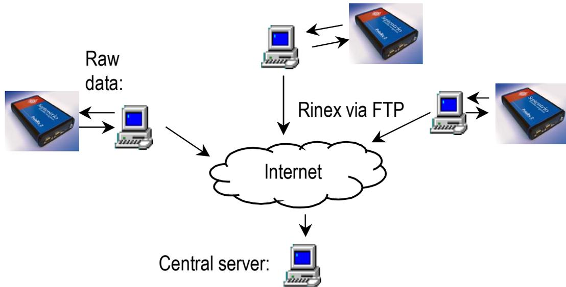
**Figure 6. Classical architecture of the data center application.**
