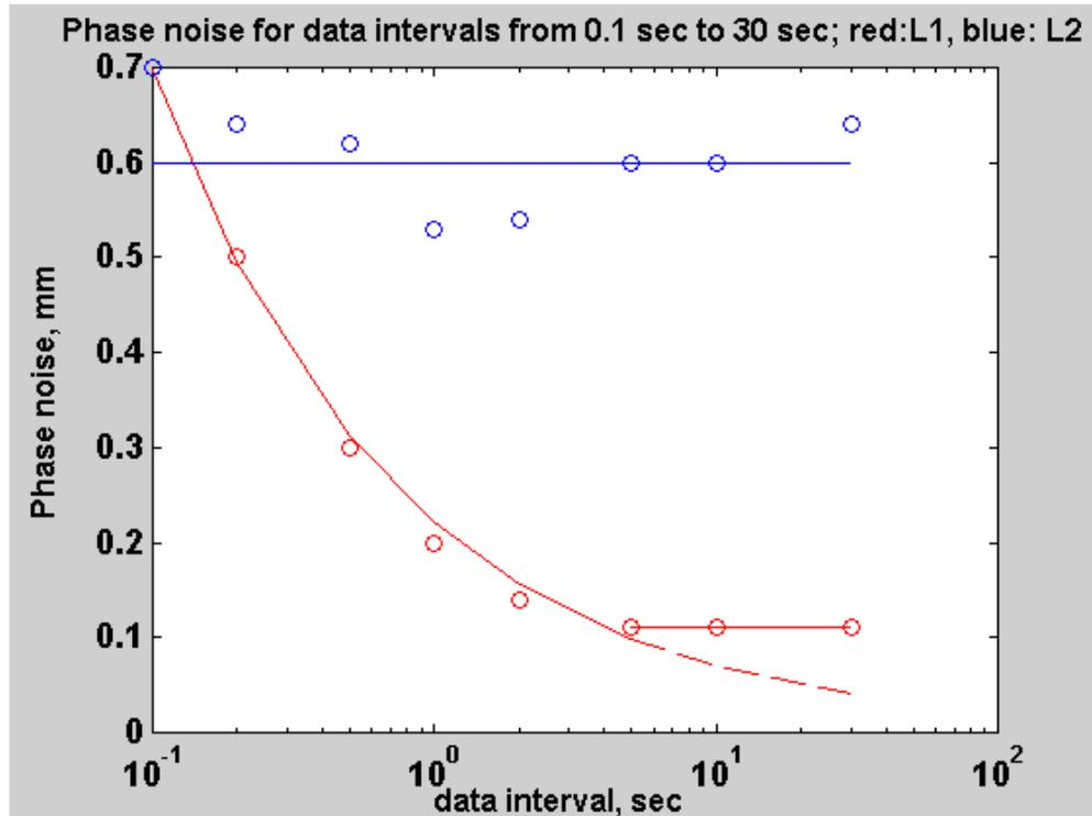
Figure 8. Tracking noise of L1 and L2 phases for data intervals from 0.1 to 30 seconds at a signal-to-noise ratio of 43 dB-Hz, representative of an average power level for actual GPS data.
