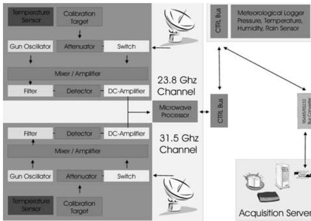
Figure 2: Technical design of the WVR of Brussels. The grey boxes represents the two High Frequency Parts of the WVR. Everything inside the left yellow box is temperature stabilized.
