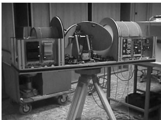
Figure 1: Picture of the generation III Water Vapor Radiometer jointly built by the Swiss Federal Institute of Technology and the CAPTEC GmbH.
