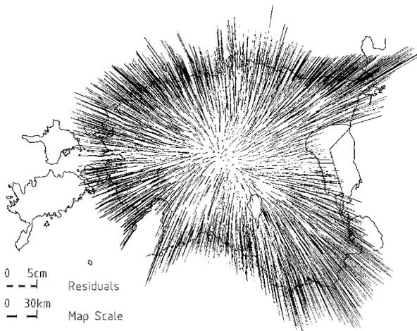
Fig. 11. Residuals of the 6 parameters HELMERT transformation, no scale difference estimated.
