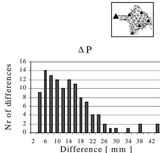
Fig. 14. The point displacements in plane between two constrained network adjustments with included  $L_1$  alone and balanced solutions, respectively.
