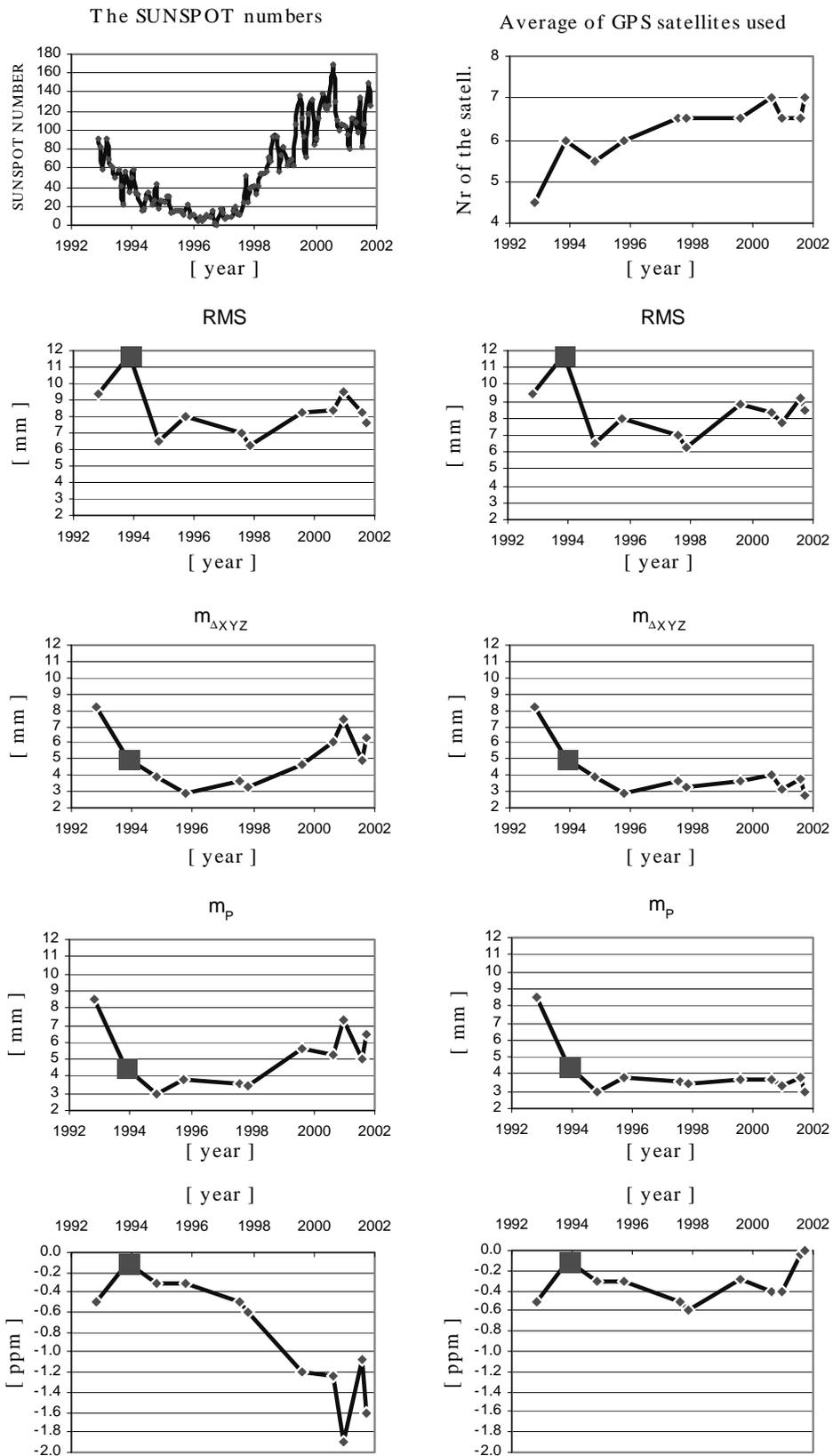
Fig. 8. The monthly average SUNSPOT numbers, average of GPS satellites used (right and left in the top), formal accuracies of the vector solutions (RMS), repeatability, a posteriori absolute accuracy from the network adjustment and the estimated scale difference between the Densification and I, II order networks (from top to bottom).  $L_1$  solutions (left) and balanced solutions implemented from year 1999 upward (right). With square the  $L1c/Widelane$  solution is denoted.
