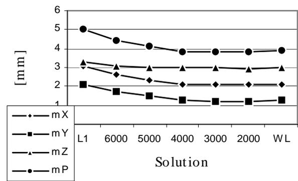
Fig. 6. Scatter of a posteriori absolute accuracy including  $L_1$ , Widelane and balanced solutions.
