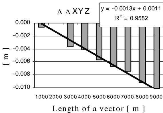
Fig. 3. Differences in length of vectors as  $L_1$  minus Widelane solution.
