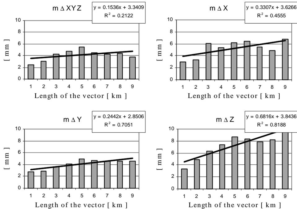
Fig. 15. The overall repeatability of vector components based on 6112 vectors measured twice or more.
