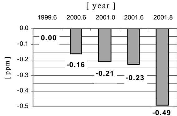
Fig. 10. The differences between the scale distortions as from comparison with higher order net minus from comparison between  $L_1$  alone and Widelane vectors.
