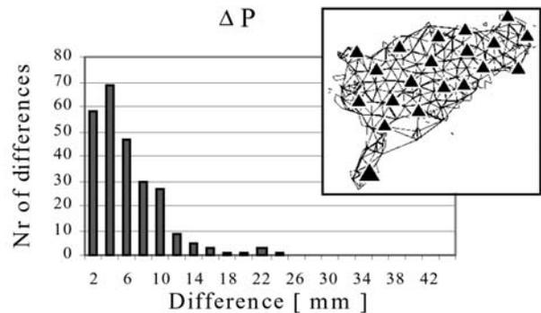
Fig. 13. The point displacements in plane between two constrained network adjustments with included  $L_1$  alone and balanced solutions, respectively.
