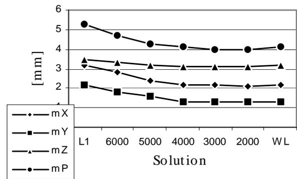
Fig. 5. Scatter of a posteriori relative accuracy including  $L_1$ , Widelane and balanced solutions.
