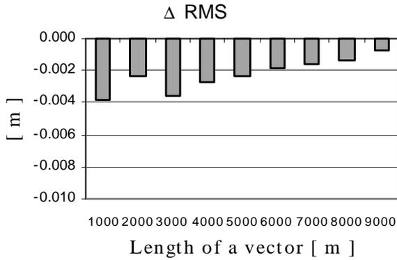
Fig. 2. Scatter of the formal accuracy as  $L_1$  minus Widelane solution
