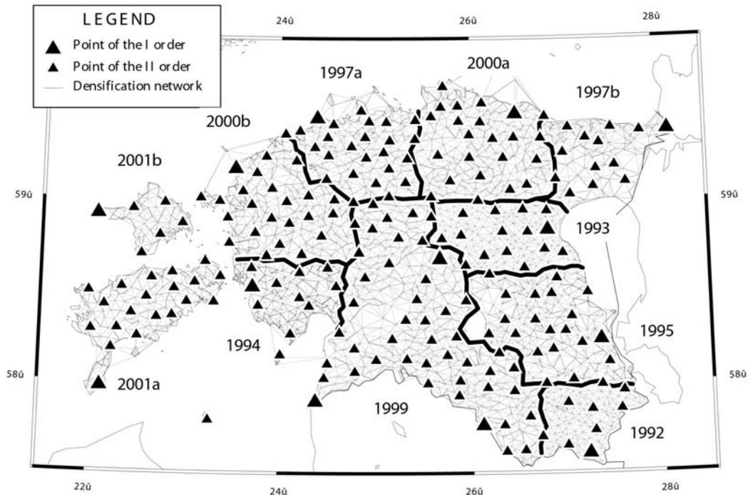
Figure 1. The Densification Network of Estonia and the years of the establishment.
