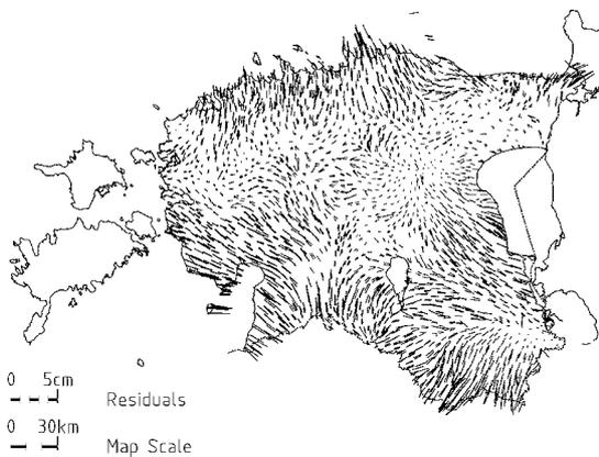
Fig. 12. Residuals of the 7 parameters HELMERT transformation, scale difference estimated.
