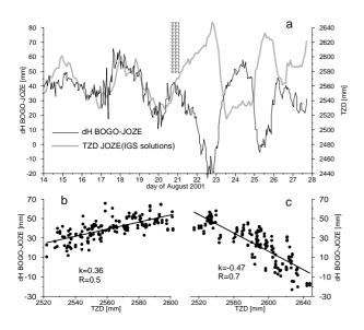
Fig. 2. Change of correlation of TZD and height variations to anti-correlation after the rainfall in August 2001
