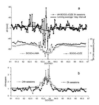
Fig. 4. Variations of the estimations of height components (a), as an eventual consequence of the internal errors in GPS data processing (b)
