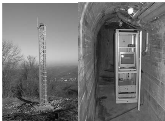
Fig. 3 Example of AGNES permanent GPS station (antenna installed on mast founded in bedrock; computer rack)
