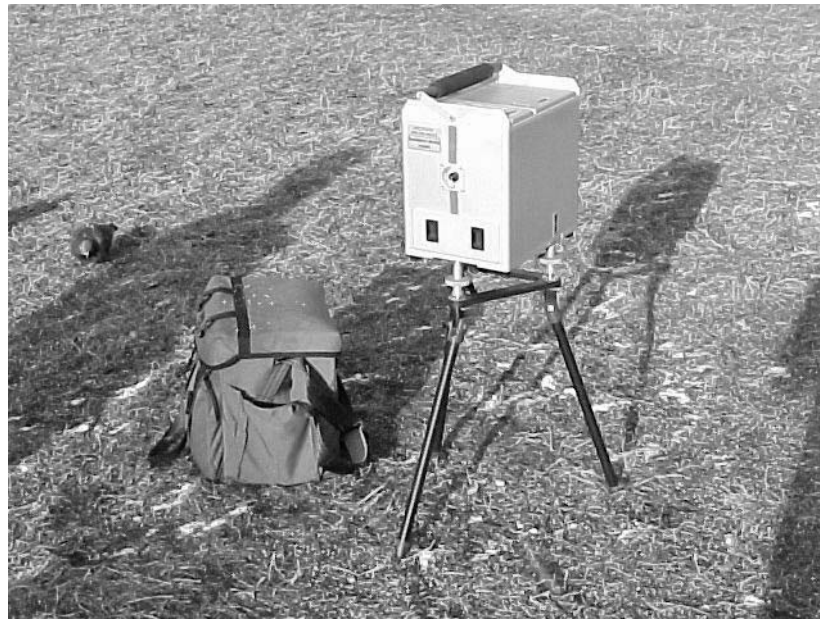
Fig. 9: Gravimeter CG – 3 in operation
