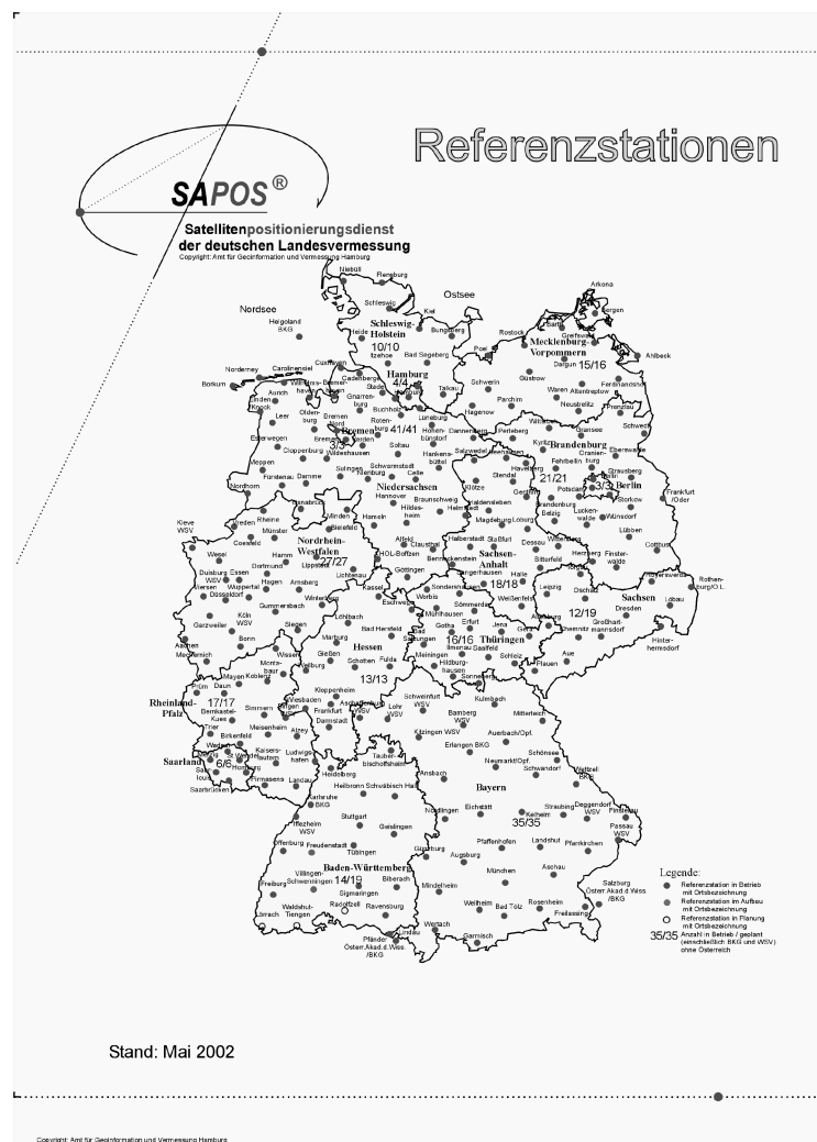
Fig. 2: Overview of the SAPOS® reference stations in the Federal Republic of Germany
