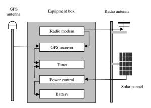
Fig. 1: Remote GPS station DMAN consisting of a GPS antenna, radio antenna, solar panel and an equipment box containing the GPS receiver and other electrical devices
