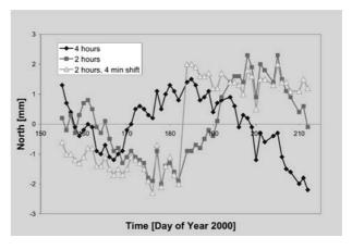
Fig. 6: Repeatability (north component) of the 60 m baseline ANDE-DMAN (section "A") for L1 solutions based on a different selection of observation intervals (4 hours, central 2 hours, 2 hours shifted by 4 minutes every day)
