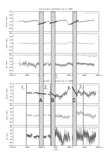
Fig. 5 indicates in which way the data of sections "A", "B" and "C", each 60 "sessions" long, were analyzed. From the available 4 hours of data different solutions were processed. One solution used all 4 hours of data, a second solution used
