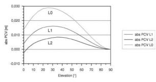
Figure 2: Elevation dependent absolute phase center correction for the Dorne Margolin AOAD/M\_T (L1, L2 and LC Signal) based on the IGS offsets.
