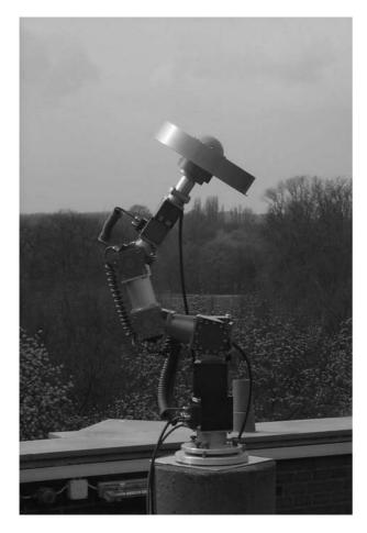
Figure 1: Robot for real time antenna calibration with test antenna.
