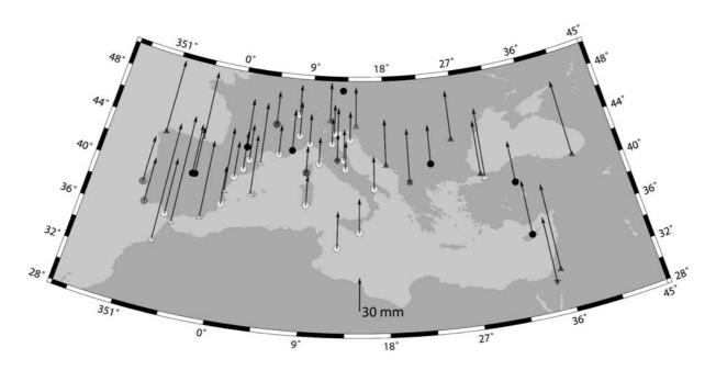
Figure 5: Apparent vertical position changes caused by absolute PCV
