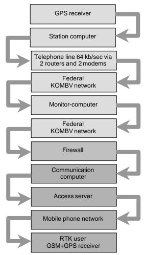
Fig. 1: Flow of GPS data from the reference receiver to the rover receiver
