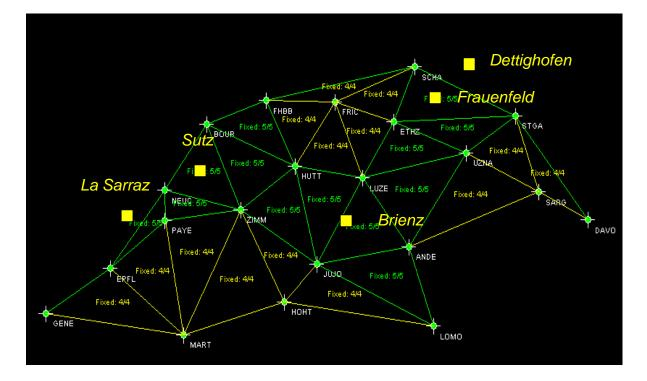
Fig. 2: Status of the AGNES RTK network. The sites Dettighofen, Frauenfeld, Brienz, Sutz and La Sarraz are used for performance tests.
