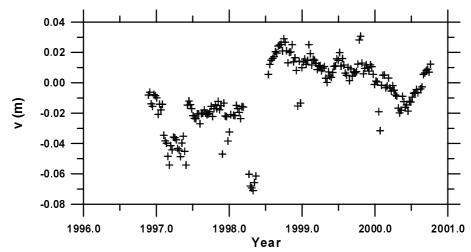
Evolution of the height component of MOPI from 1996.8 to 2000.8 (jumps are due to radome manipulations and reference frame changes)
