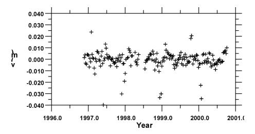
Evolution of height component of MOPI after introduction correction due to radome manipulations
