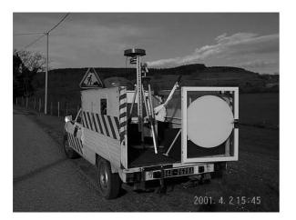
Equipment used to make levelling with GPS
