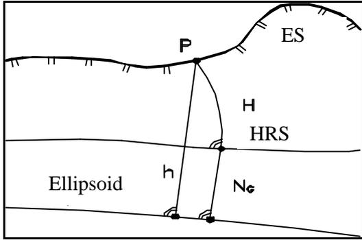
**Fig. 1:** Ellipsoidal GPS height  $h$ , standard height  $H$ , height reference surface HRS, its ellipsoidal height  $N_G$  and earth surface ES at a point  $P(B,L)$
