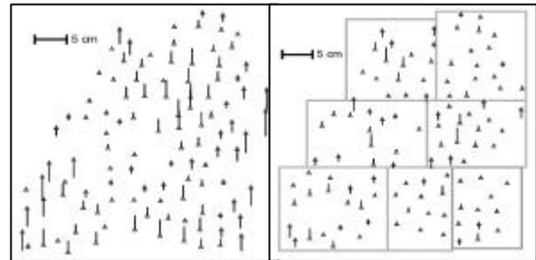
**Fig. 4:** Effect of a "geoid-patching" at the example of Baden-Württemberg: Large residuals in identical points with only one set of datum parameters (left) and much smaller residuals with 7 patches with individual datum sets  $\partial N_G(\mathbf{d}^j)$  (right).
