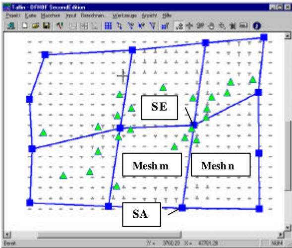
**Fig. 2:** Irregular mesh grid and different observation types (geoid data grid; triangles meaning identical points  $(H,h)$ ). Example of DFHRS data base computation of Tallinn, Estonia with DFHRS production software.
