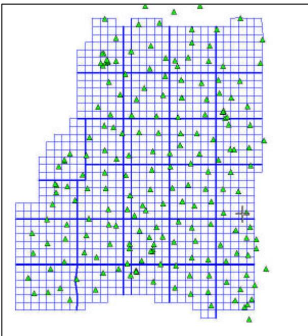
**Fig. 5:** DFHRS production for the country of Baden-Württemberg, Germany. Area size 250 km x 350 km. Almost regular meshes with an average size of 7 km, 28 geoid-patches, 1013 meshes and 192 identical points.
