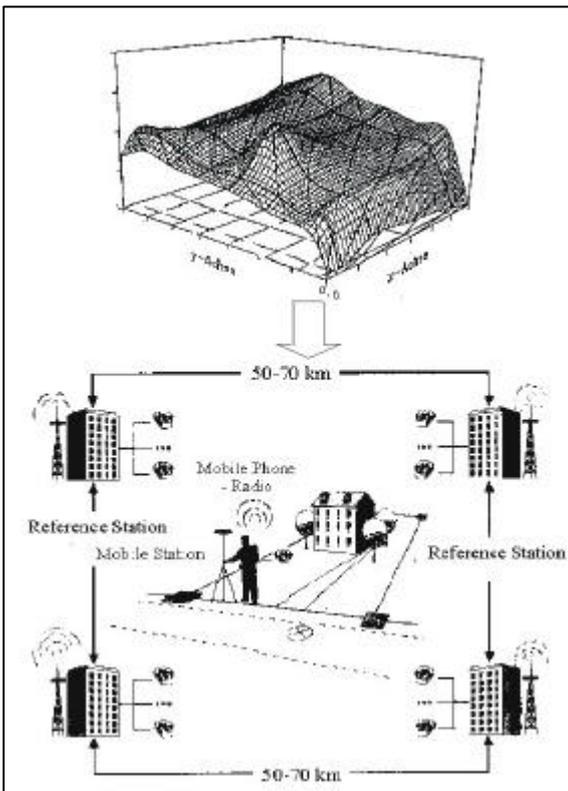
**Fig. 3 :** DFHRS data base symbolized by the Finite Element Model  $N_{FEM}(\mathbf{p})$  of the HRS (above) and "application scenery" of an online GPS-heighting (below).
