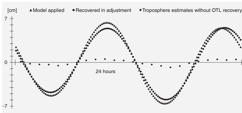
Fig. 7 Applied vertical ocean tide loading displacement at ACOR on day 231, 1997 and recovery by harmonic functions.
