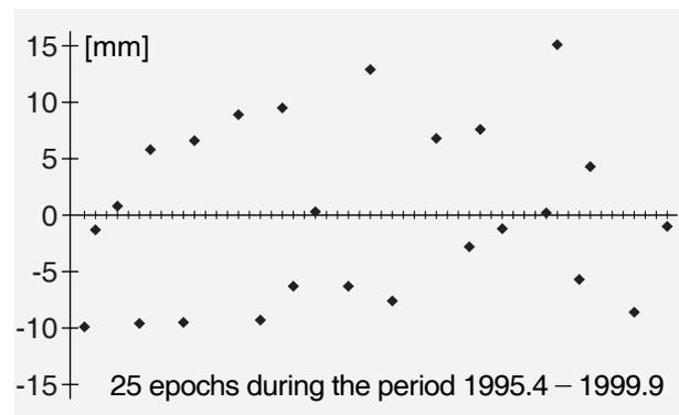
Fig. 5: Time series of the ellipsoidal height difference on baseline BRST-MAS1: errors due to not modeling ocean tide loading in the adjustment.
