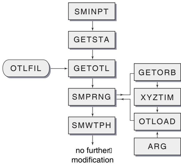
Fig. 1: Extension of the Bernese simulation program to apply site displacements due to ocean loading.
