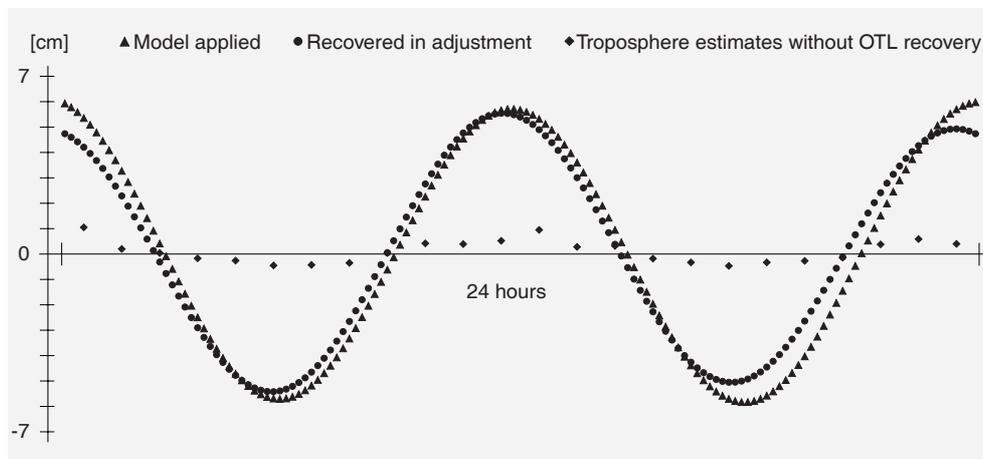
Fig. 6 Applied vertical ocean tide loading displacement at BRST on day 270, 1995 and recovery by harmonic functions
