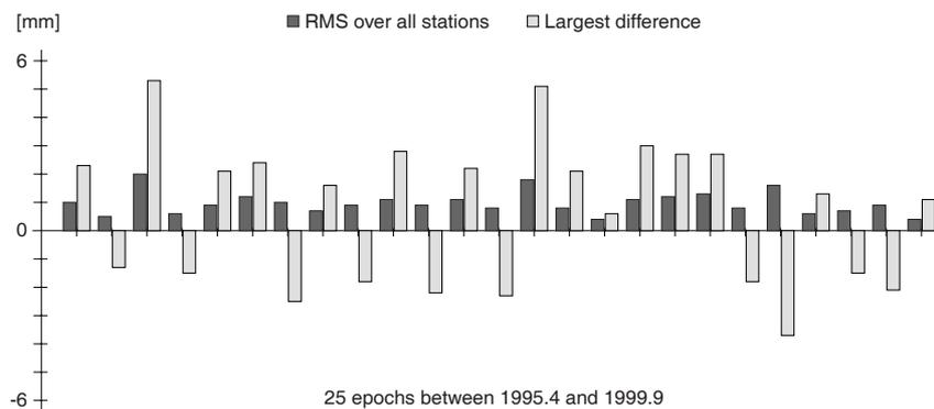
Fig. 4: Differences between height estimates from daily network adjustments with and without modeling ocean tide loading.
