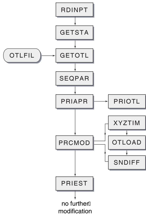
Fig. 2: Modification of the Bernese adjustment program to apply site displacements due to ocean loading and/or to model it by harmonic functions.
