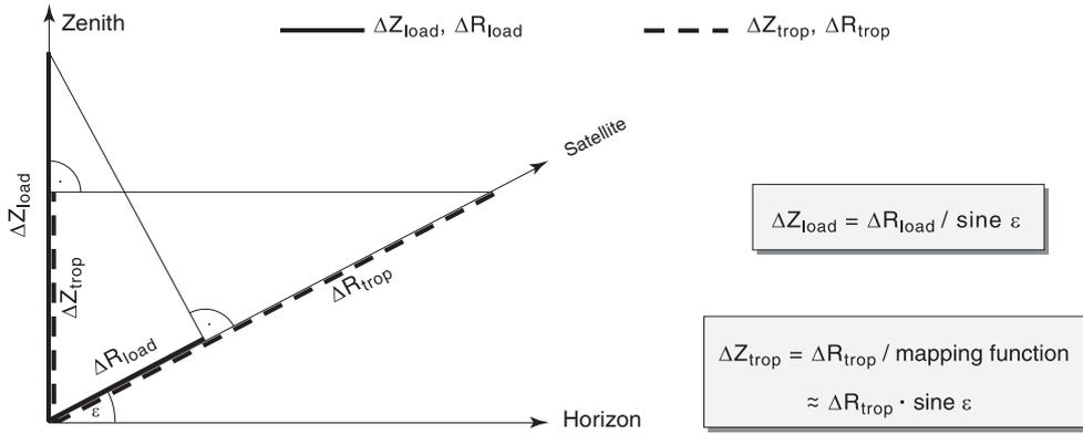
Fig. 3: Separation of vertical loading displacements and tropospheric delays.
