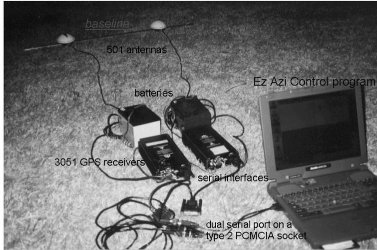
Fig. 1 the setup of the breadboard attitude/heading sensor.
