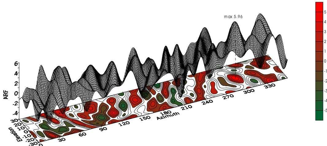
Fig. 2: Example of structure in the Azimuth-elevation space of the ambiguity function, with seven satellites. The maximum is correctly identified at (Az,El) = (292.5°, -0.3°)
