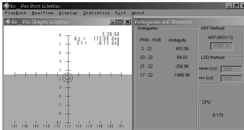
Fig. 3: Windows based interface providing status of the solution and information on time, satellites and position. The integer status of the ambiguities can be checked at each instant.
