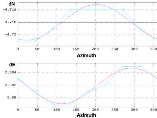
Figure 3. Phase center position changes of antenna RA0033 for L1 frequency in m (broken line is observation result, smoothed line is harmonical approximation)
