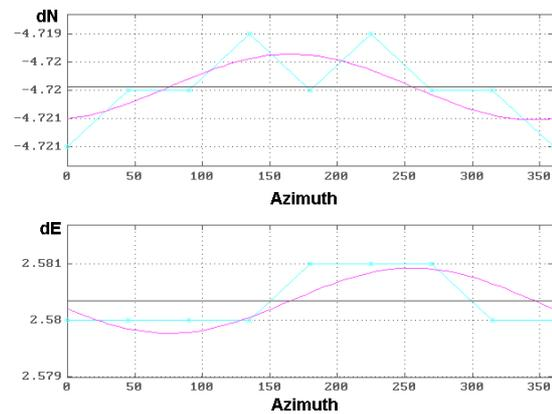
Fig.4. Phase center position changes of antenna RA0023 for L2 frequency in m (broken line is observation result, smoothed line is harmonical approximation)
