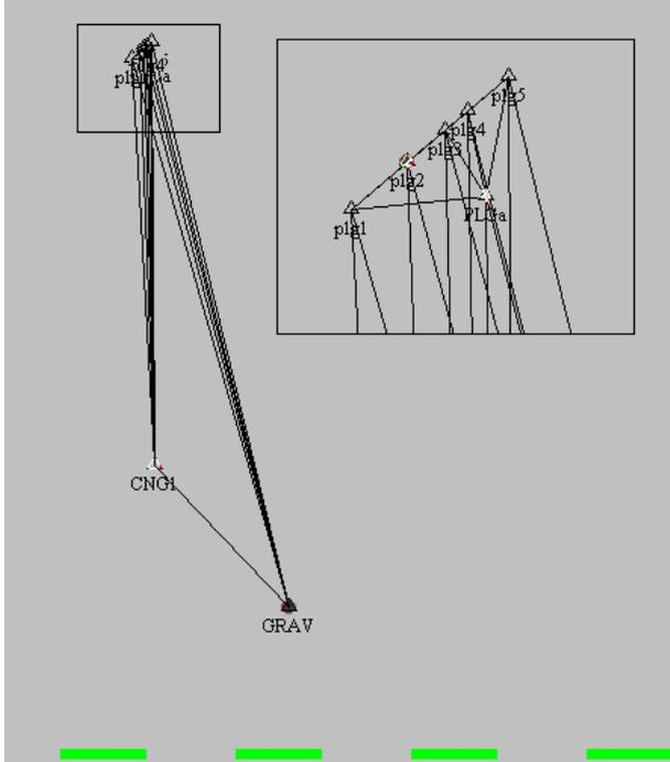
Fig.2. Expanded terrestrial control network (large scale fragment shows standard baseline and astronomic point)
