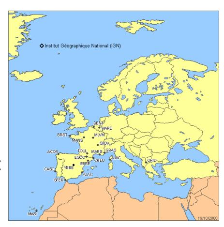
Based on these GPS permanent Stations and with other additional equipments for broadcasting and data links to a control centre, a new project to provide necessary data for a real-time positioning on the decimetre level was launched this year. The IGN, in cooperation with other governmental organisations will be responsible for the deployment and the exploitation of this network.
