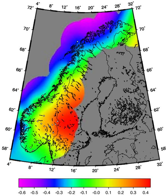
Fig. 2: The difference between the models VREF1996 and NKG96n (units meter) and the adjustmentpoints used when computing VREF1996.
