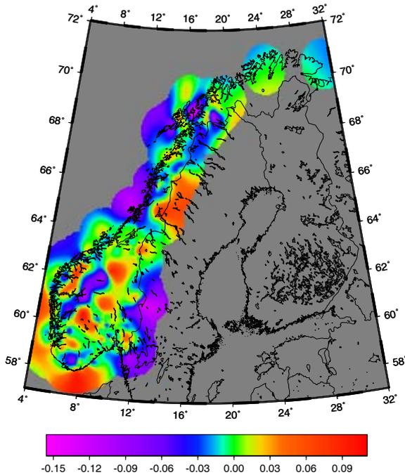
Fig. 4: The geoid difference between the GPS/levelling data set and VREF2000b (units meter)
