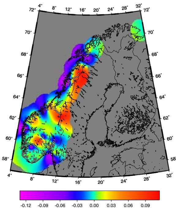
Fig. 3: The difference between the models VREF1998 and VREF1996 (units meter) and the adjustmentpoints used when computing VREF1998.
