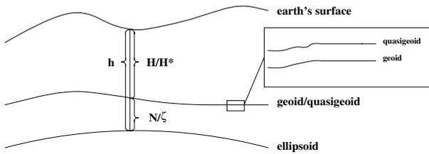
Fig. 1: The relationship between the geoid, the quasigeoid, geoid height, height-anomaly, orthometric height and normal height.
