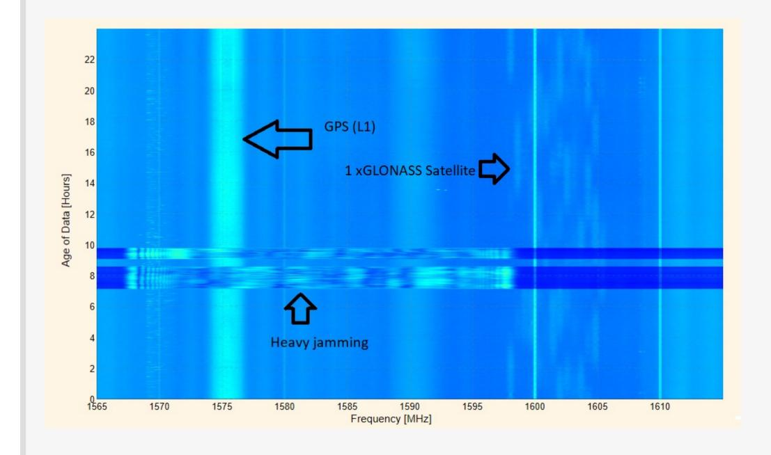
OS Net raw GNSS spectrum data feeds are integrated with OS Net RTCM data. The spectrum data analysis is automated using machine learning and AI techniques to automatically recognise, alert for and categorise interference events.
