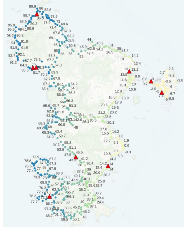
Fig. Left) Difference btw levelling campaigns 2006 and 2023. No gravity correction applied. Right) Model prediction.
