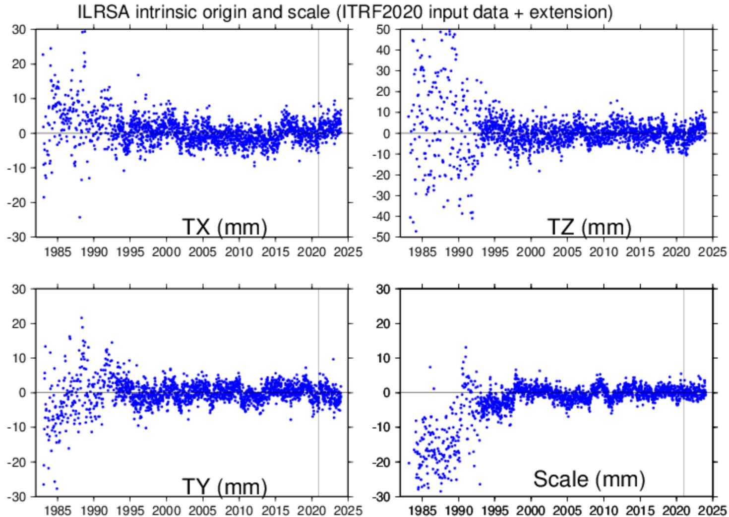
SLR Origin & scale accuracy at 2015.0 below 1 mm and scale stability at the level of 0.1 mm/yr
