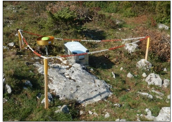
Figure 5: 72-hour static GNSS survey at the SOCE (Socerb) geodynamic site in October 2022
