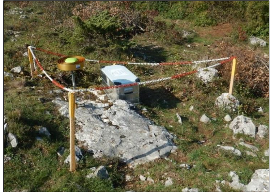
Static GNSS survey at the Socerb geodynamic site
