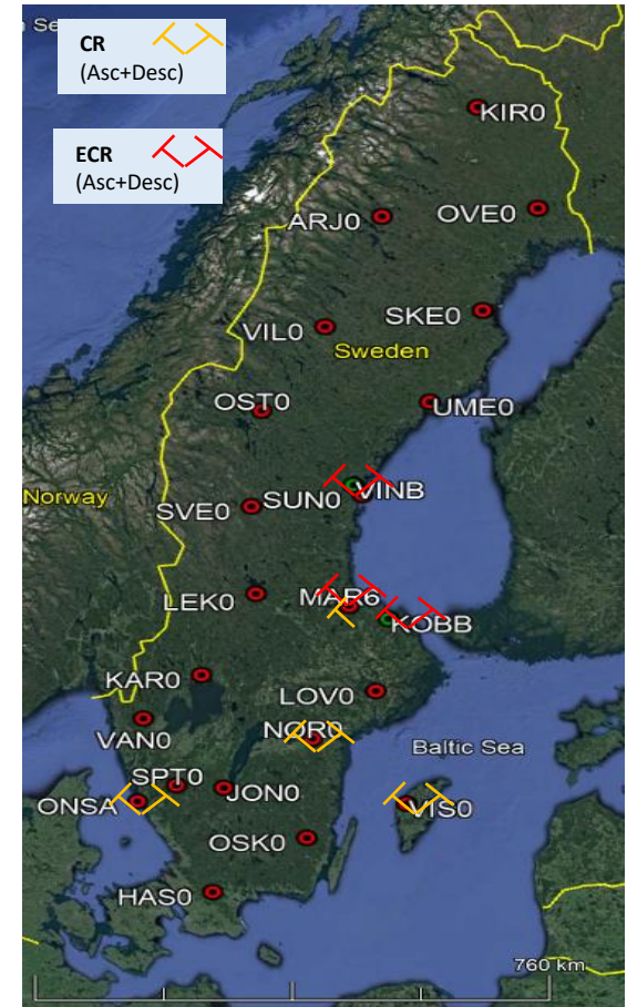
GNSS fundamental stations (red circles) and current CR/ECR installations
