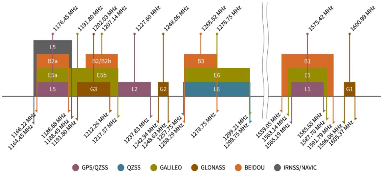
**Fig. 1** Frequencies used by the main global and regional navigation satellite systems (source [www.tallysman.com](http://www.tallysman.com)).
