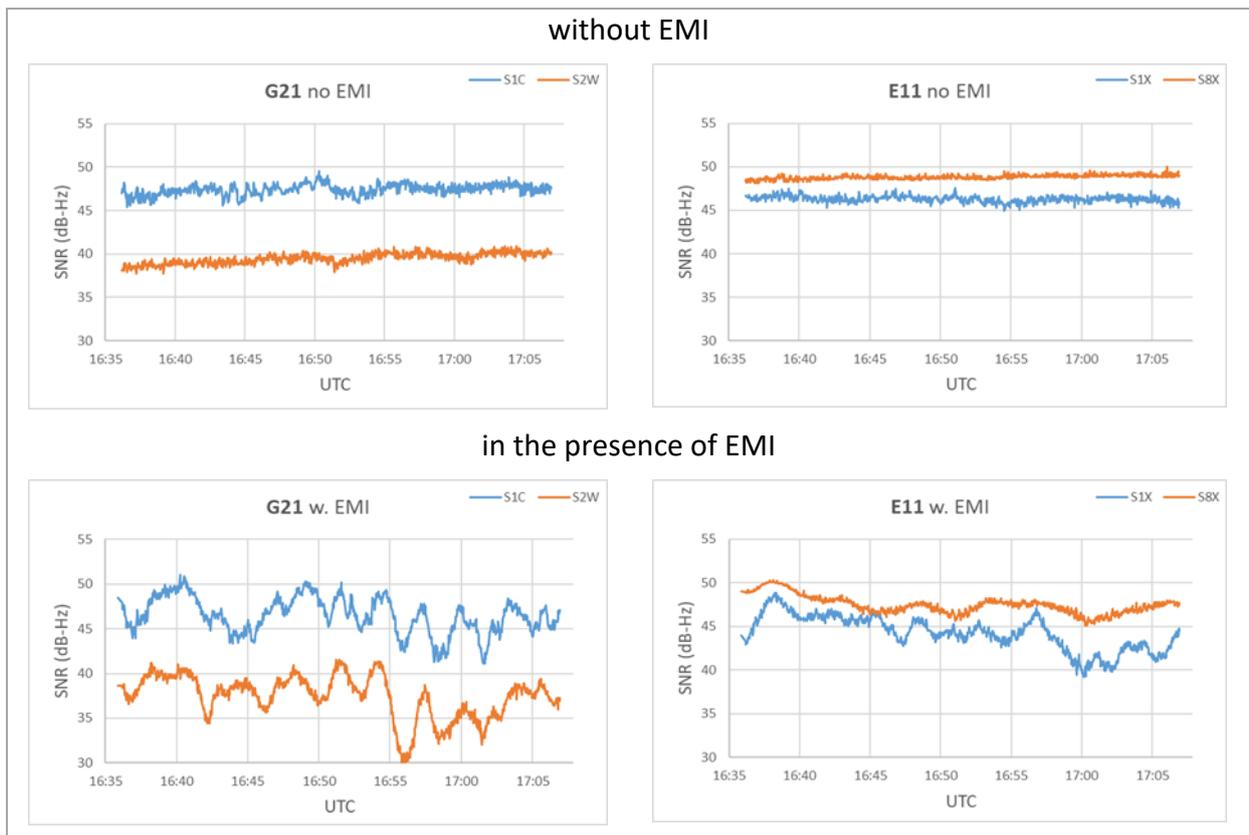
**Fig. 12** Case 1b: SNR comparison between GPS and GAL with and without EMI. Primary frequencies (L1, E1) are marked blue; Secondary frequencies (L2, E5) are marked orange.
