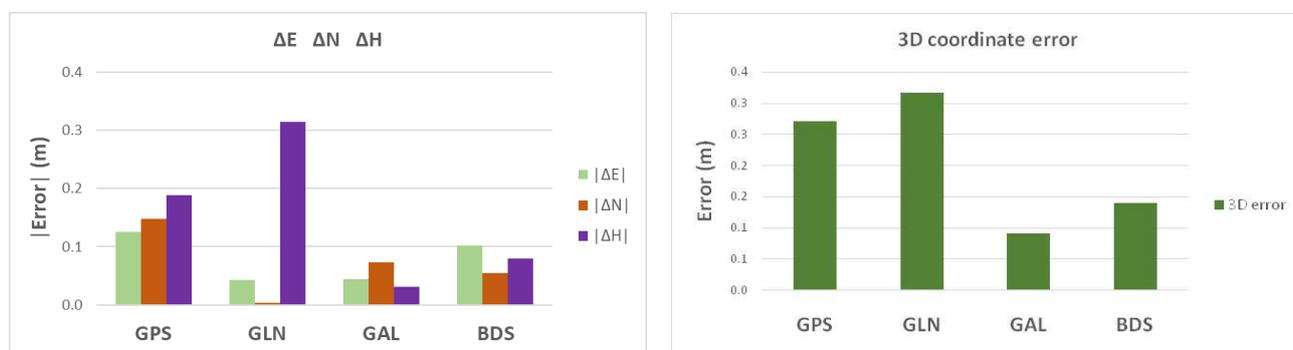
**Fig. 5** Case 1a: Comparison of coordinate errors among GPS, GLN, GAL and BDS:  $\Delta E$ - $\Delta N$ - $\Delta H$  (left) and 3D error (right).
