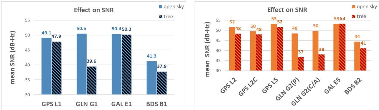
**Fig. 8** Case 2a: SNR comparison between GPS, GLN, GAL and BDS in open sky and under tree canopies for the primary frequencies (left, in blue) and the secondary frequencies (right, in orange).
