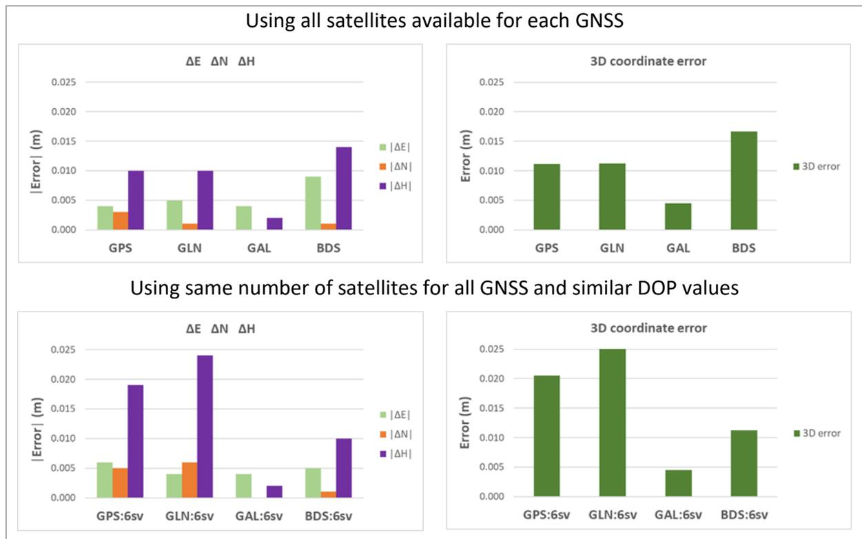
**Fig. 17** Case 2b: Comparison of coordinate errors among GPS, GLN, GAL and BDS:  $\Delta E$ ,  $\Delta N$  and  $\Delta H$  (left) and 3D error (right).
