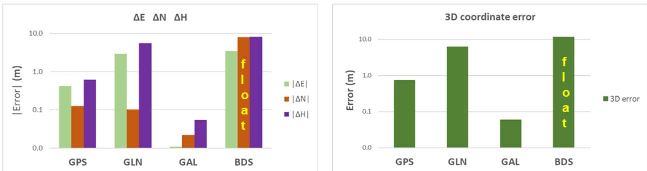
**Fig. 9** Case 2a: Comparison of coordinate errors among GPS, GLN, GAL and BDS:  $\Delta E$ - $\Delta N$ - $\Delta H$  (left) and 3D error (right).
