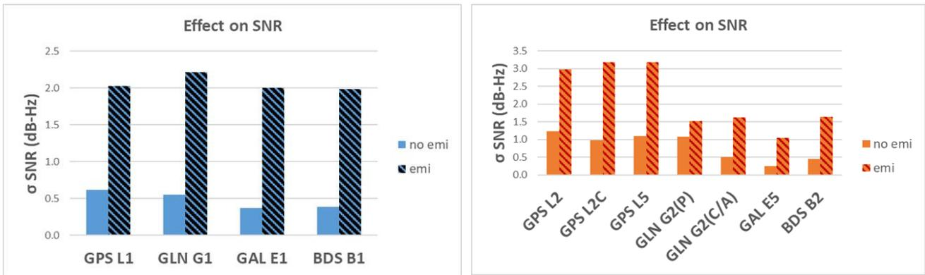
**Fig. 15** Case 1b: SNR comparison between GPS, GLN, GAL and BDS with and without EMI for the primary frequencies (left, in blue) and the secondary frequencies (right, in orange).
