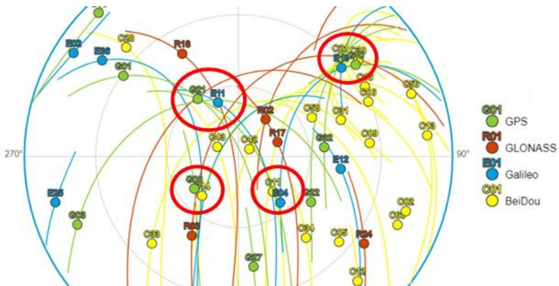
**Fig. 2** Detail from a sky plot showing satellites that can be compared (marked with red circles).
