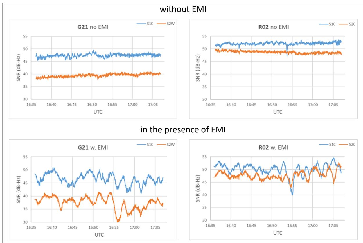
**Fig. 11** Case 1b: SNR comparison between GPS and GLN with and without EMI. Primary frequencies (L1, G1) are marked blue; Secondary frequencies (L2, G2) are marked orange.
