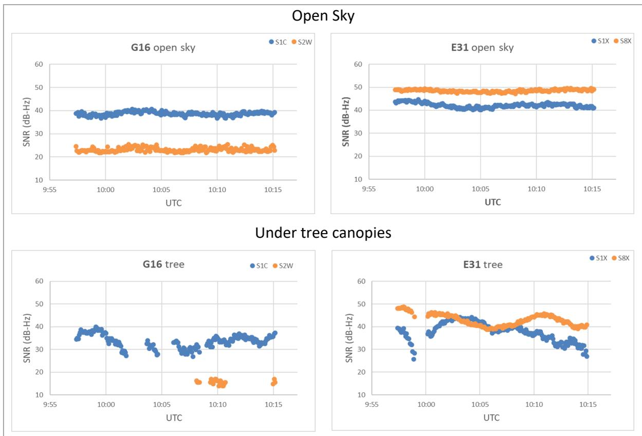
**Fig. 4** Case 1a: SNR comparison between GPS and GAL in open sky and under tree canopy. Primary frequencies (L1, E1) are marked blue; Secondary frequencies (L2, E5) are marked orange.
