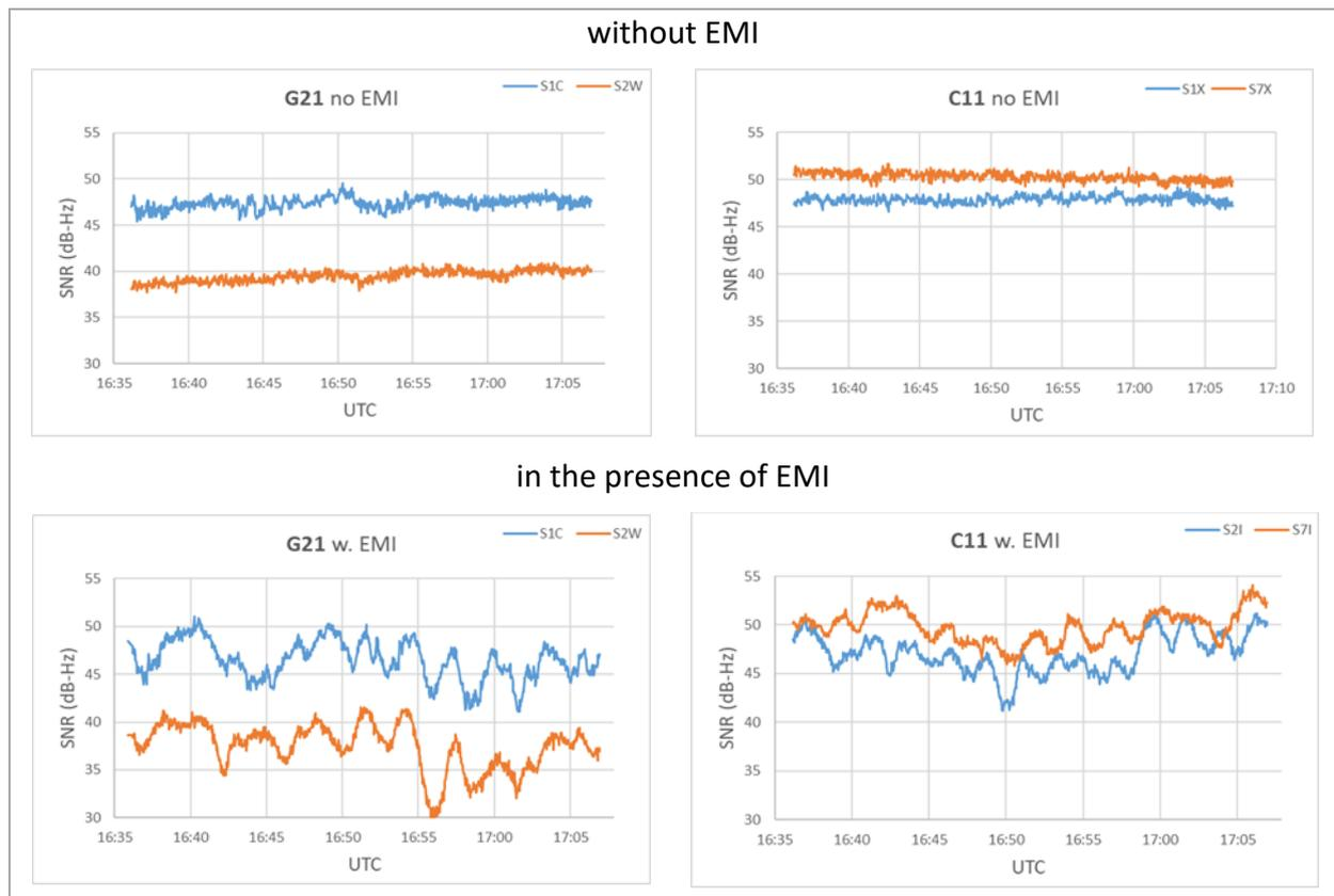
**Fig. 14** Case 1b: SNR comparison between GPS and BDS with and without EMI. Primary frequencies (L1, B1) are marked blue; Secondary frequencies (L2, B2) are marked orange.
