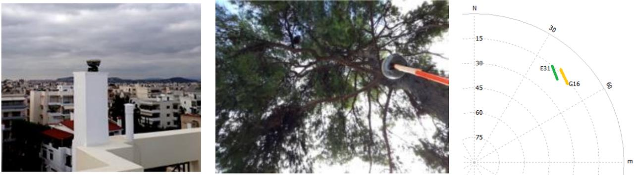
**Fig. 3** Case 1a: Base in open sky (left), rover under canopy (middle) and paths of the satellites under comparison (right).
