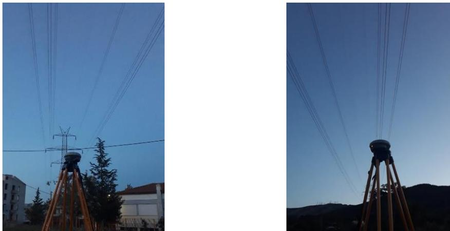
**Fig. 16** Case 2b: Location of the rover under the power lines.
