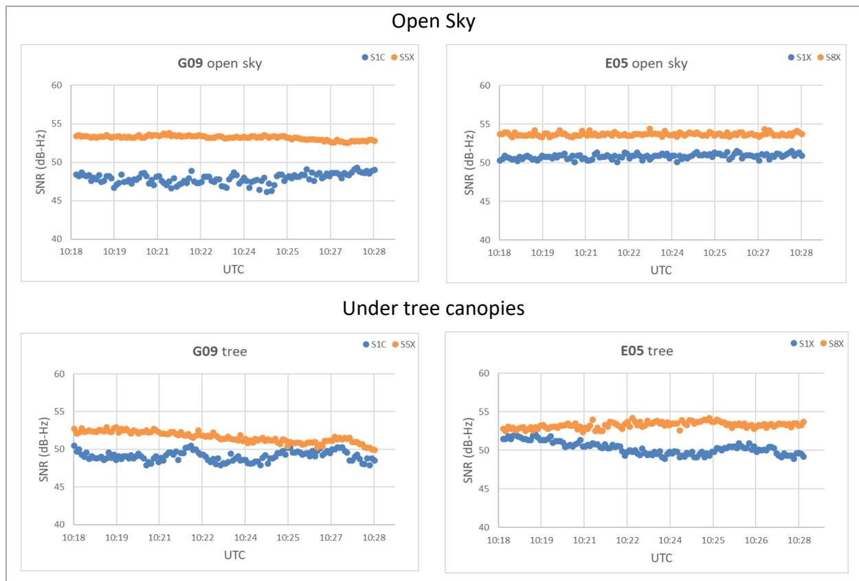
**Fig. 7** Case 2a: SNR comparison between GPS and GAL in open sky and under tree canopy. Primary frequencies (L1, E1) are marked blue; Secondary frequencies (L5, E5) are marked orange.
