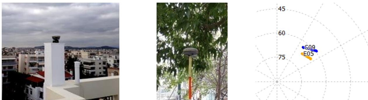
**Fig. 6** Case 2a: Base in open sky (left), rover under canopy (middle) and paths of the satellites under comparison (right).
