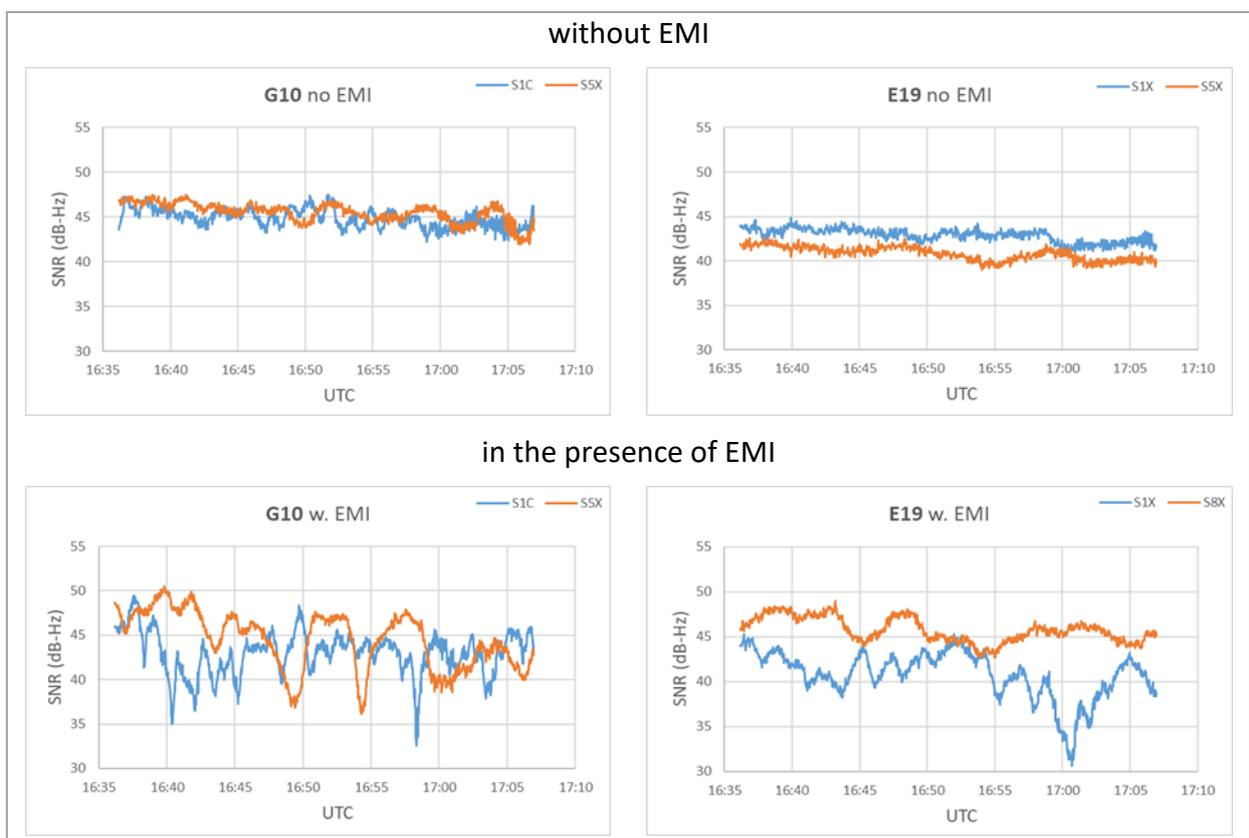
**Fig. 13** Case 1b: SNR comparison between GPS and GAL with and without EMI. Primary frequencies (L1, E1) are marked blue; Secondary frequencies (L5, E5) are marked orange.
