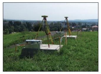
Figure 4: A pair of passive GNSS control points.
