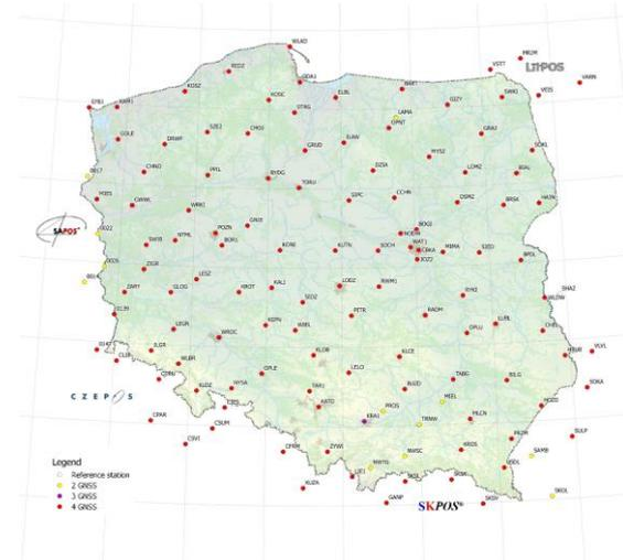
Fig. 36. Reference stations of the ASG-EUPOS system (March 2021)
