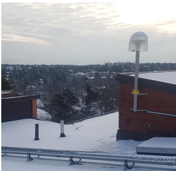
Figure 4.2: Gustavsberg is a SWEPOS class B station with a roof-mounted GNSS antenna established mainly for network RTK purposes.
