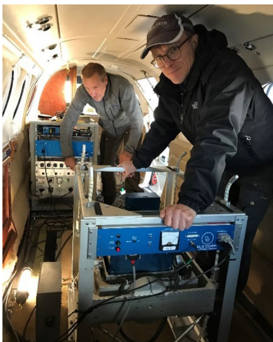
Figure 9.1: The airborne Kattegat campaign in October 2018: Installation of Lantmäteriet's ZLS dynamic gravity meter TM in the airplane.
