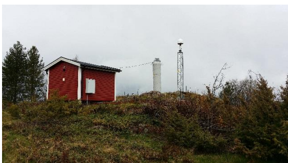
Figure 4.1: Sveg is one of the SWEPOS stations belonging to class A. It has both a new monument (established in 2011) and an old monument (from 1993).
