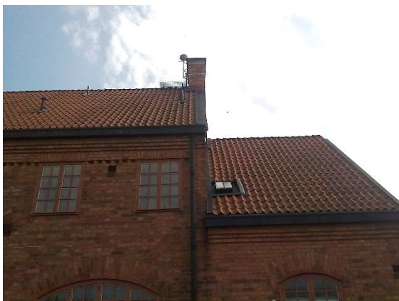
Figure 4.2: Vagnhärad is a class B SWEPOS station with a roof-mounted GNSS antenna mainly established for network RTK purposes.
