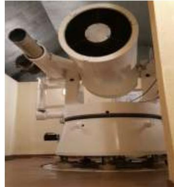
Fig. 41. Second independent satellite laser system developed by SRC PAS (main telescope)
