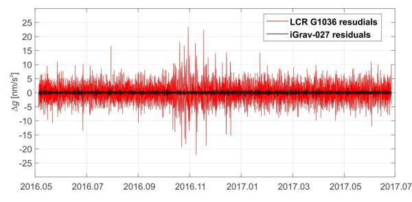
residuals from tidal adjustment with the use of high pass filter
