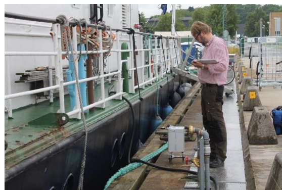
Figure 9.1: Harbour tie gravity measurement made by Lantmäteriet in the FAMOS project.
