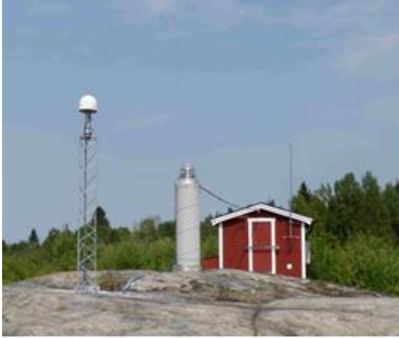
Figure 4.1: Hässleholm is one of the SWEPOS stations belonging to class A. It has both a new monument (established in 2011) and an old monument (from 1993).
