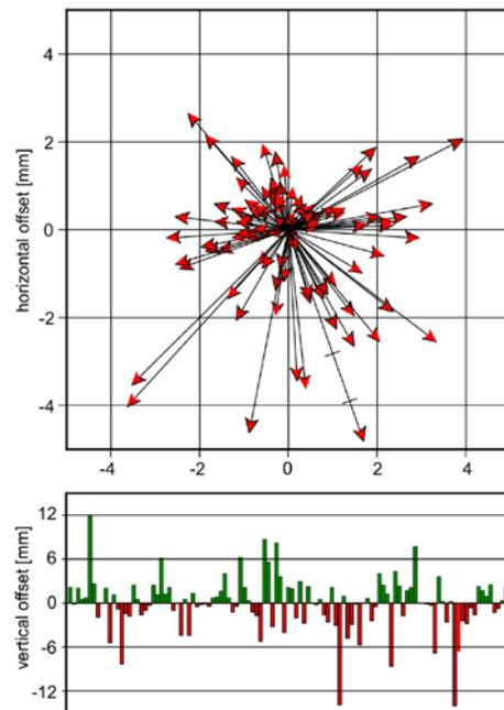
Fig. 9. Position offsets related to mixing type mean and individual antenna phase centre corrections; each arrow/column refers to one antenna-radome mounted at one station (stations in alphabetical order)
