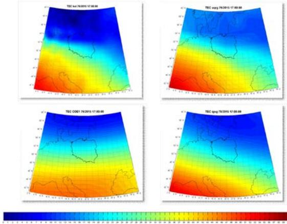
Fig. 19. Comparison between the ionosphere maps derived using the new regional TEC model UWM-rc1, IGS, COE and UQRG model for the active day (17 March 2015)
