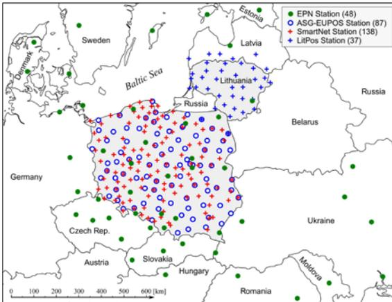
Fig. 17. GNSS network processed by the WUELS AC in NRT mode for troposphere parameter estimation
