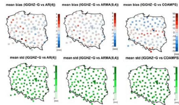
Fig. 16. Mean biases and standard deviations from residuals  $ZTD_{IGGHZ-G} - ZTD_{model}$ , where 'model' is one of the following: AR(4), ARMA(8,4) or COAMPS for 121 ASG-EUPOS stations; data are averaged between 1.12.2012 – 15.03.2013
