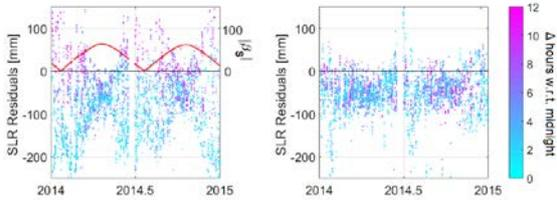
Fig. 11. SLR residuals to Galileo-102 as a function of the local time of collected data at a station. Daytime observations are shown in magenta, whereas night time observations in cyan. Left figure is generated using classical ECOM, whereas the right one using extended ECOM (for the same satellite)
