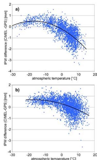
Fig. 14. IPW difference (CIMEL-GPS) for Thule-THU2 for 2009–2011 a) and Ittoqqortoormiit – Scoresbysund (SCOR) for 2012–2014 b) as a function of atmospheric temperature, IGS tropospheric solution
