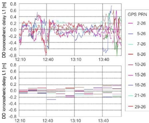
Fig. 24. Double-differenced ionospheric delays on L1 frequency for TREO-LYNS baseline obtained from geometry-free solution with fixed ambiguities for original observations (top) and RTC-corrected observations (bottom) (Sieradzki and Paziewski, 2015a)
