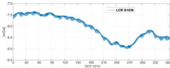
Fig. 28. Gravity record with LCR-G gravimeter in Borowa Gora Observatory averaged in 1 hour window
