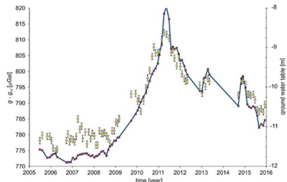
Fig. 1. Absolute gravity surveyed with the FG5-230 at Jozefoslaw (100 cm height) ( $g_{\text{ref}} = 981213000 \mu\text{Gal}$ )
