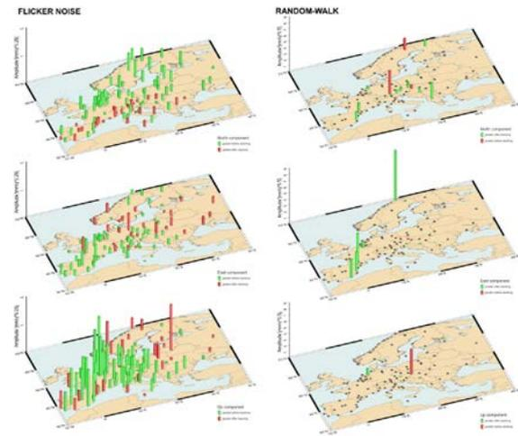
Fig. 32. Amplitudes of flicker (left) and random-walk (right) processes for selected EPN network stations' time series before and after filtering with stacking; the plots correspond to (from the top) North, East, Up components, respectively; the green colour represents a decrease in noise amplitudes when filtration was performed, whereas the red colour shows an increase which was observed mainly for short time series
