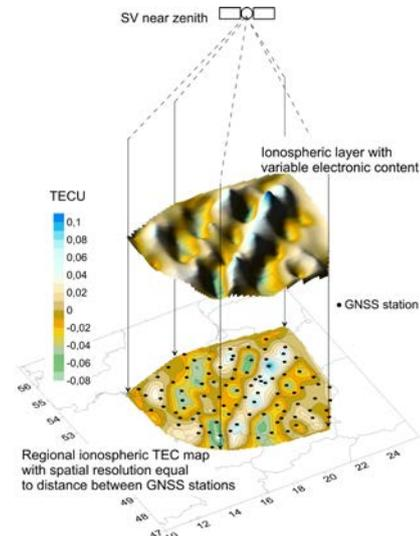
Fig. 21. Scheme of TEC mapping by the method of orthogonal parallel-beam projection
