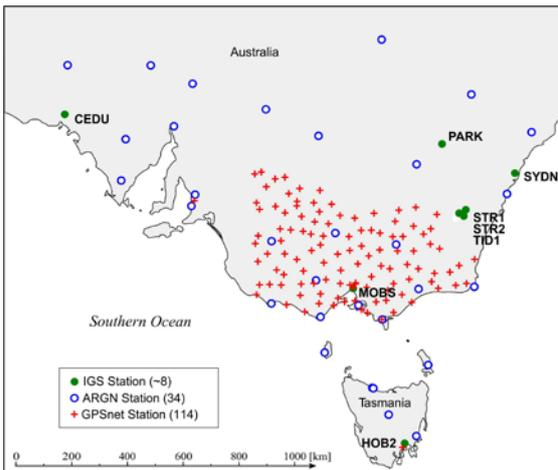
Fig. 18. GNSS network processed in NRT mode for troposphere parameter estimation by the RMIT University in cooperation with WUELS
