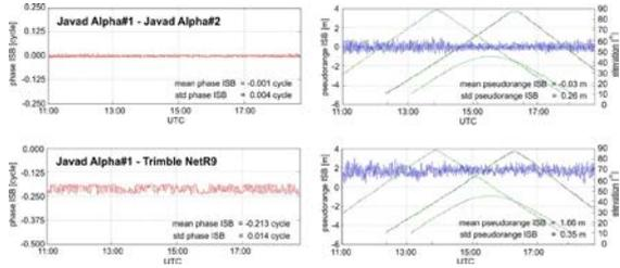
Fig. 23. Phase and code ISB time series obtained using all available GPS and Galileo satellites for different receiver pairs: 1<sup>st</sup> row – homogenous receivers (Javad Alpha), 2<sup>nd</sup> row inhomogeneous receivers (Javad Alpha – Trimble NetR9). Source: Paziewski et al. (2015)
