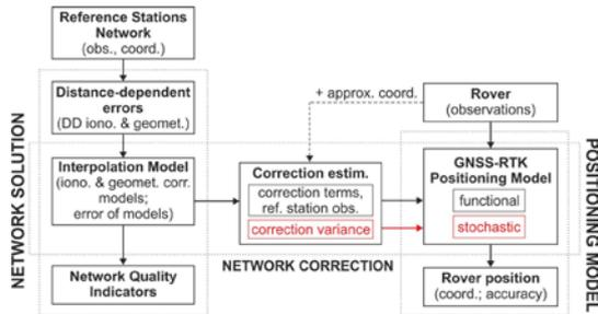
Fig. 25. Network RTK positioning model based on NBSM; in red – new elements of the model added by NBSM
