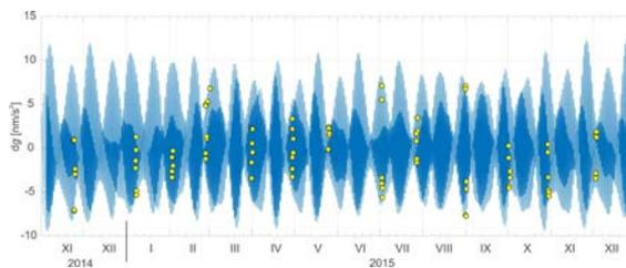
Fig. 29. Differences between local and global tidal ephemeris in 2015; differences for epochs of gravity determination with the A10-020 gravimeter marked with yellow dots
