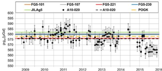
Fig. 2. Absolute gravity surveyed with the A10-020 at Borowa Gora (pillar level) ( $g_{ref} = 981125000 \mu\text{Gal}$ )
