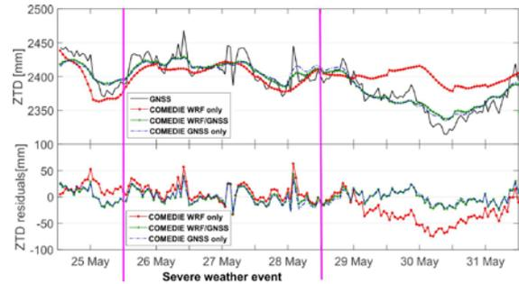
Fig. 15. Comparison of ZTD from GNSS station KRAW with ZTDs from COMEDIE from 3 data sets: WRF only (red), WRF/GNSS (green) and GNSS only (blue) (top) with corresponding residuals of  $ZTD_{GNSS} - ZTD_{COMEDIE}$  [mm] for all data sets (bottom); data period 25 – 31 May 2014
