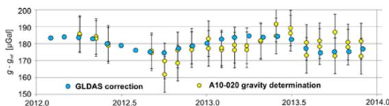
Fig. 3. Regular monthly absolute determinations of gravity on field station at Borowa Gora Observatory with respect to GLDAS hydrological model correction ( $g_{ref} = 981\,250\,000 \mu\text{Gal}$ )
