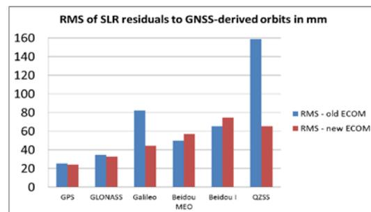
Fig. 10. Mean RMS of SLR residuals to GNSS-derived orbits [mm]; validation of orbits from 2010–2013 (GPS+GLONASS) and 2014 (Galileo+BeiDou+QZSS) is shown
