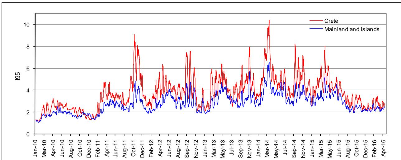
**Fig. 5** Mean daily I95 index estimated from HEPOS (values are smoothed using moving average filtering).
