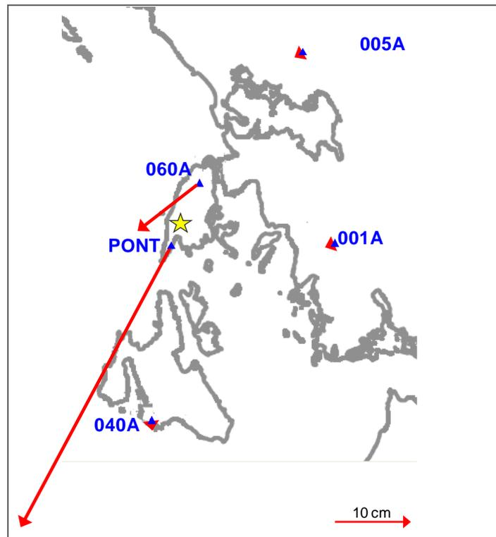
**Fig. 10** Estimated static horizontal displacements at five reference stations. The epicentre of the earthquake is marked by yellow star.
