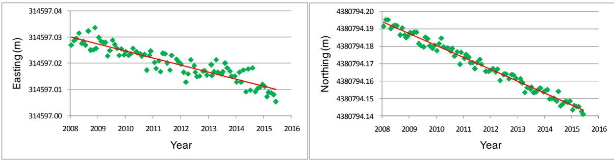
**Fig. 1** Time-series for Easting (left) and Northing (right) of HEPOS station 071A in Thessaly.
