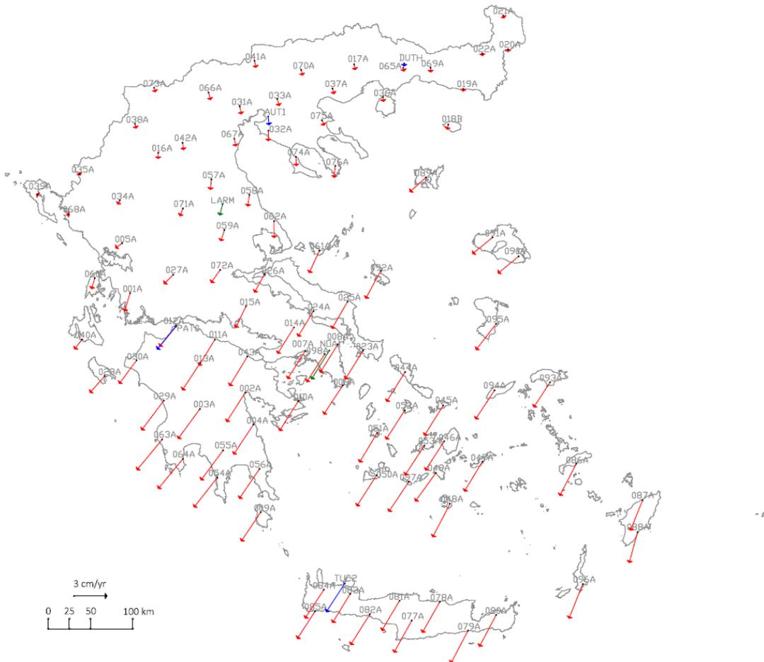
**Fig. 3** Estimated horizontal velocities in ETRF2000 for HEPOS stations (red arrows) and EPN Class B stations (green arrows). For comparison reasons the velocities published by EUREF for the EPN Class A stations are also shown (blue arrows).
