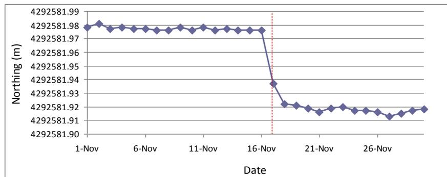
**Fig. 9** Time-series of Northing of station 060A (the vertical dashed line indicates the day of the earthquake).
