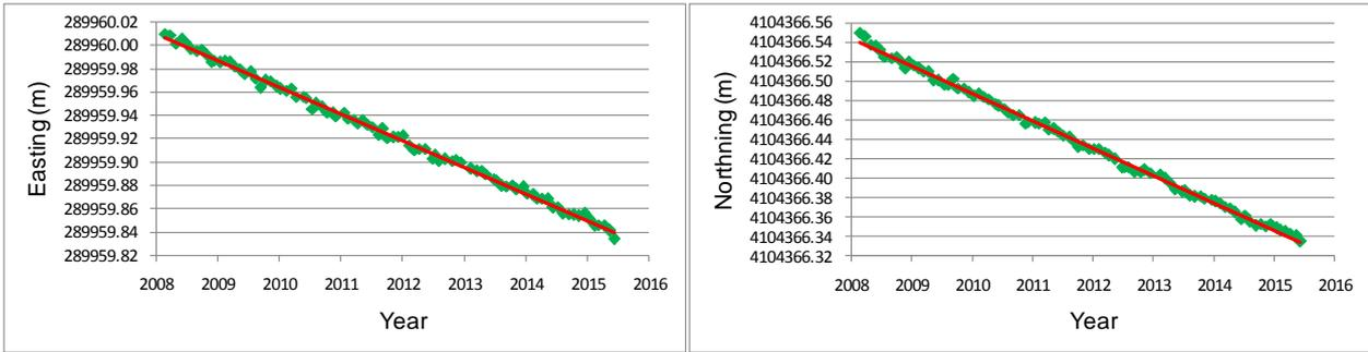
**Fig. 2** Time-series for Easting (left) and Northing (right) of HEPOS station 063A in Peloponnese.
