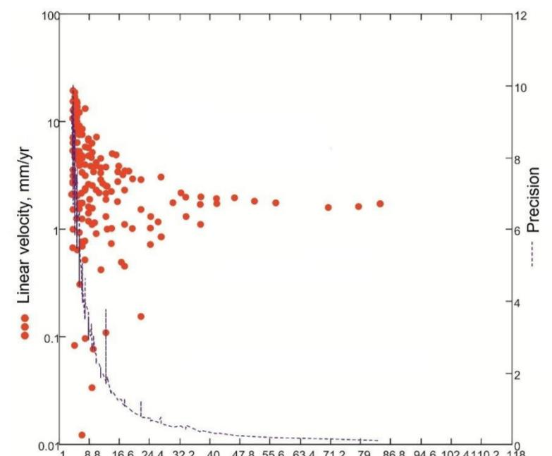
Fragment of calculation results  $V_{TG}$  and  $m_{V_{TG}}$  depending on the duration of observations on the example of Travemunde tide gauge (Germany)
